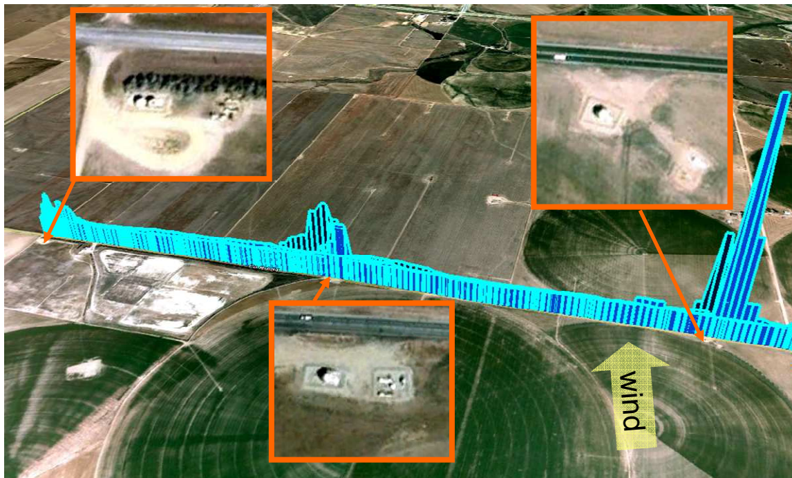
Figure 1: Localization of fugitive emissions from multiple production pads
