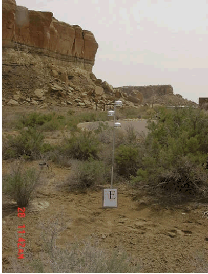
Figure 2. PSDs mounted on metal pole.
