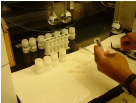
Figure 5. Preparation for analysis: (a) pad removal, (b) sonication, and (c) transfer to autosampler tubes.
