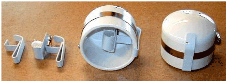
Figure B-1. Plastic clips and protective shelter for the Ogawa passive sampler (photo courtesy Ogawa and Co., USA Inc.).
