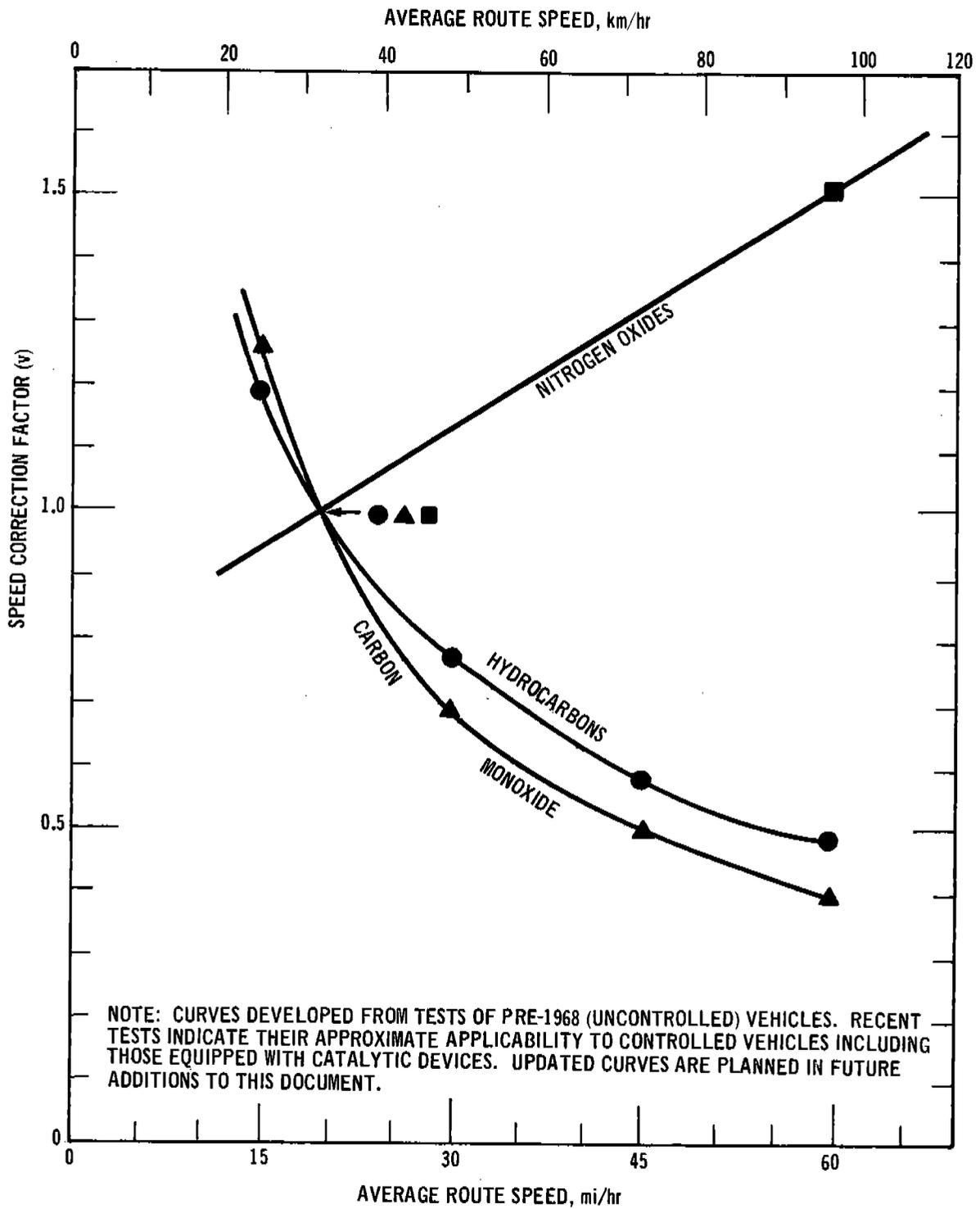
Figure 3.1.1-1. Average speed correction factors for all model years.<sup>5-7</sup>
