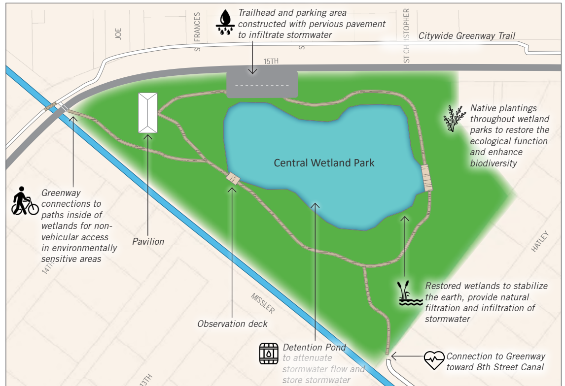
Proposed Concept for Central Wetland Park. The concept plan was prepared with assistance from the National Park Service - Rivers, Trails & Conservation Assistance Program.
