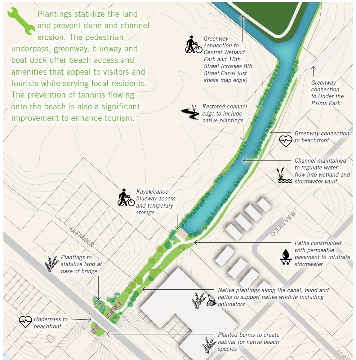
The proposed plan to end 8th Street Canal creates a pond, greenway extension and an underpass to the beachfront.
