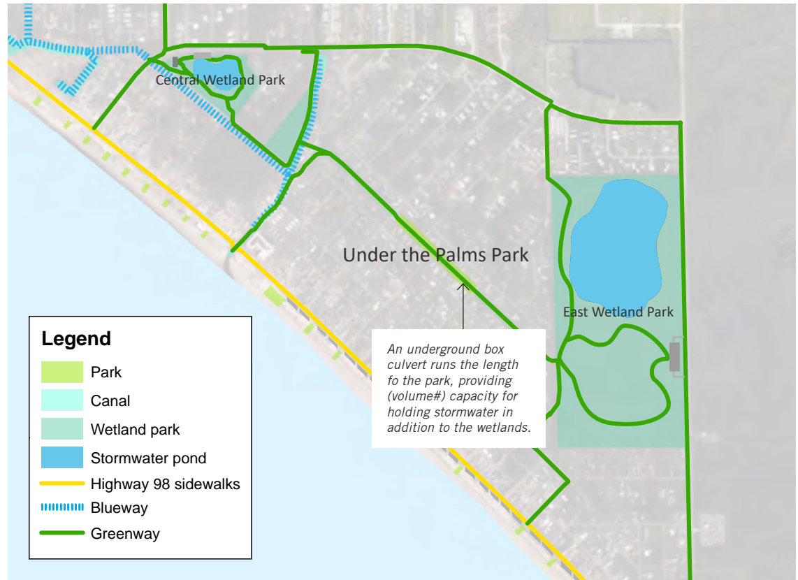
Proposed wetland parks are connected by drainage channels and an underground box culvert, significantly increasing potential water storage area.
