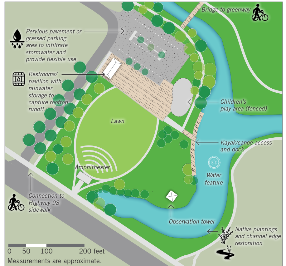
Option B plan for Parker Park closes part of the canal to enlarge entry and lawn area.
