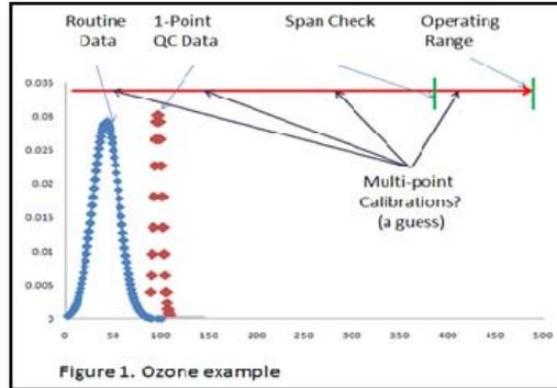
using 4 upscale points with the highest point at 450 ppb. The span check, based on guidance of 80-90% of the operating range, is at 400 ppb. The one point QC check, based on the requirement of 10 - 100 ppb, is at 90 ppb and the routine data 3-year average is about 40 ppb.
