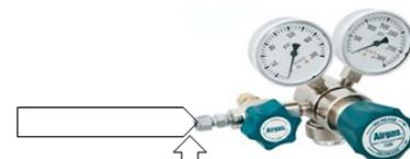
Attach a Nitrogen cylinder to purge lines!
