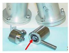
Speciation sampling canister with corrosion in cyclone.
