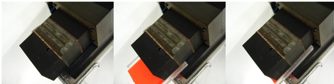
*Figure 9.2.9.2 No Spacer / Figure 9.2.9.3 Spacer half inserted / Figure 9.2.9.4 Spacer Fully Inserted*
