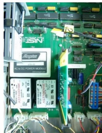
*Figure 9.2.6.1 STOLAB Card/* *Figure 9.2.6.2 STOLAB Location on MB/* *Figure 9.2.6.3 STOLAB inserted*
