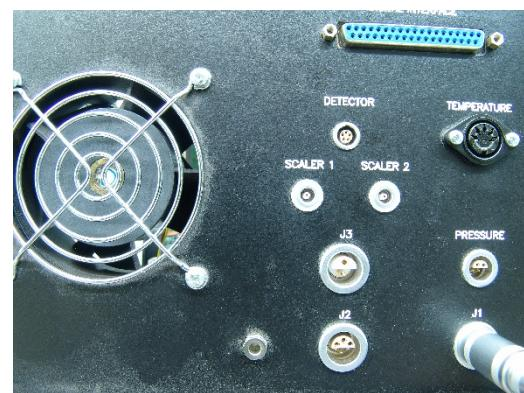
Figure 9.3.1.2 J1 Connected
