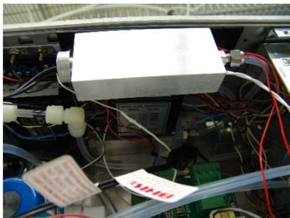
*Figure 9.2.7.3 heated block and MFC*
