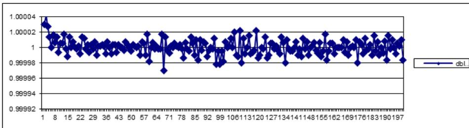
The Pass/Fail criteria are based on the last three Std. Dev. For Scalar1 and Scalar2, they should be <15 and the Std. Dev. For the three Ratios should each be <0.00003.
