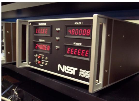
*Figure 9.3.3.9 SRP Electronics module (initial start-up)*
