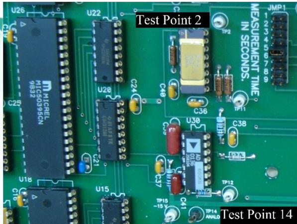
Figure 9.5.2.5.2 Close up showing TP2 and TP14
