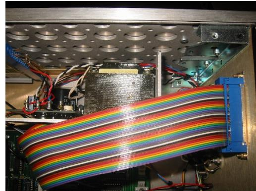
Figure 9.2.5.1 Inside the Electronics Module    Figure 9.2.5.2 Ozone Boards power supply
