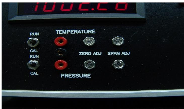
*Figure 9.5.2.6.2 Zero Adjust and Span Adjust for Pressure*
