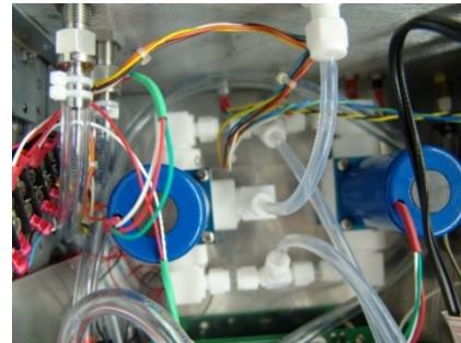
**Figure 9.2.7.1 Inside the Pneumatics Module /Figure 9.2.7.2 New style of solenoid valves**
