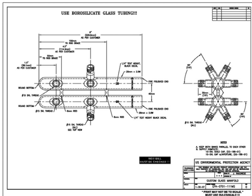
Figure 9.4.11.1 Dual glass manifold schematic
