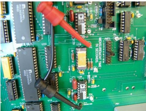
Figure 9.5.2.5.3 TP2 and TP14 connected.
