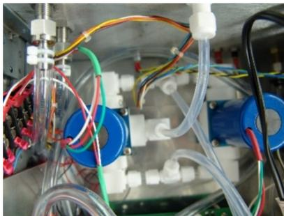
*Figure 9.2.7.1 Inside the Pneumatics Module /Figure 9.2.7.2 New style of solenoid valves*
