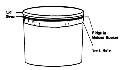
Figure 2-2. Plastic Bag Liner Assembly
