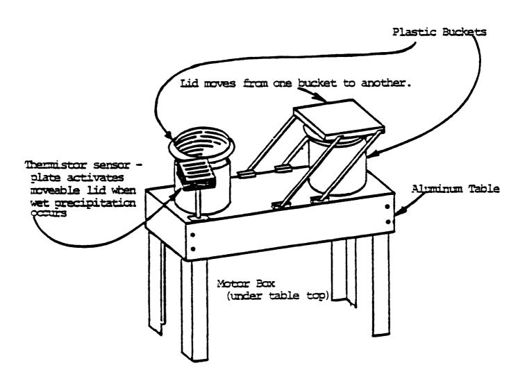
Figure 2-1. Wet/Dry Precipitation Collector
