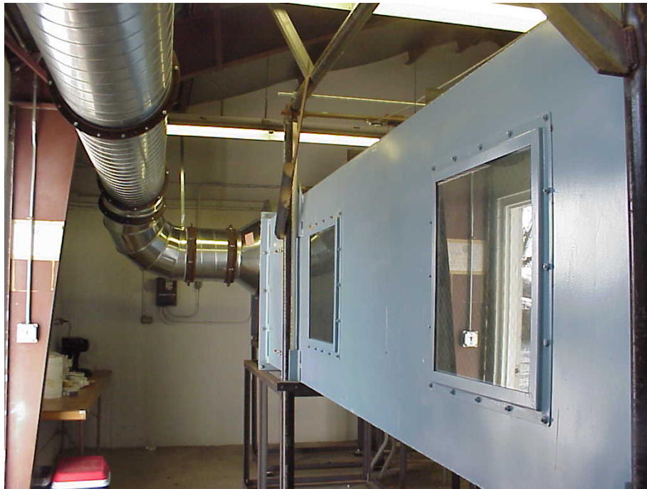
Figure 3. Return Line to Wind Tunnel Blower
