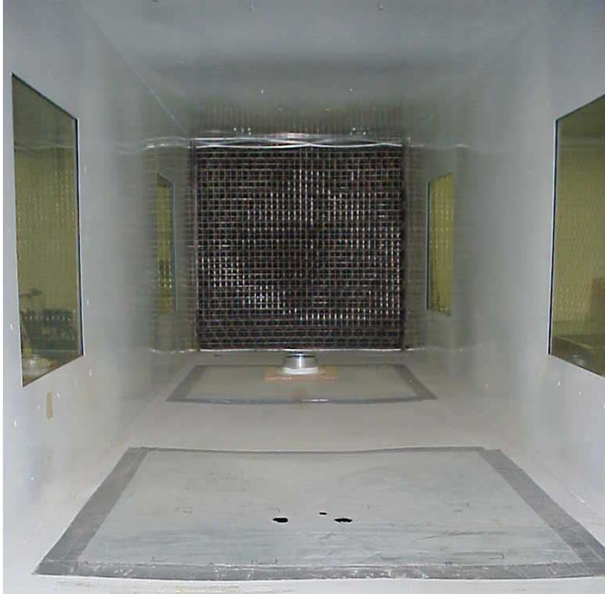
**Figure 5. Test Chamber Interior With Flow Straightener
