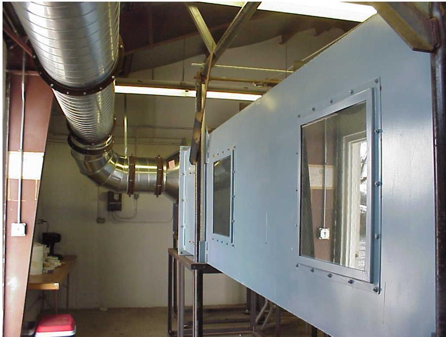
**Figure 3. Return Line to Wind Tunnel Blower**
