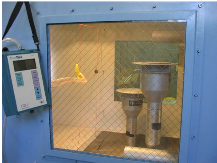
Figure 7. View of Partisol, Cyclone, and DustTrak Inlets Through Observation Window
