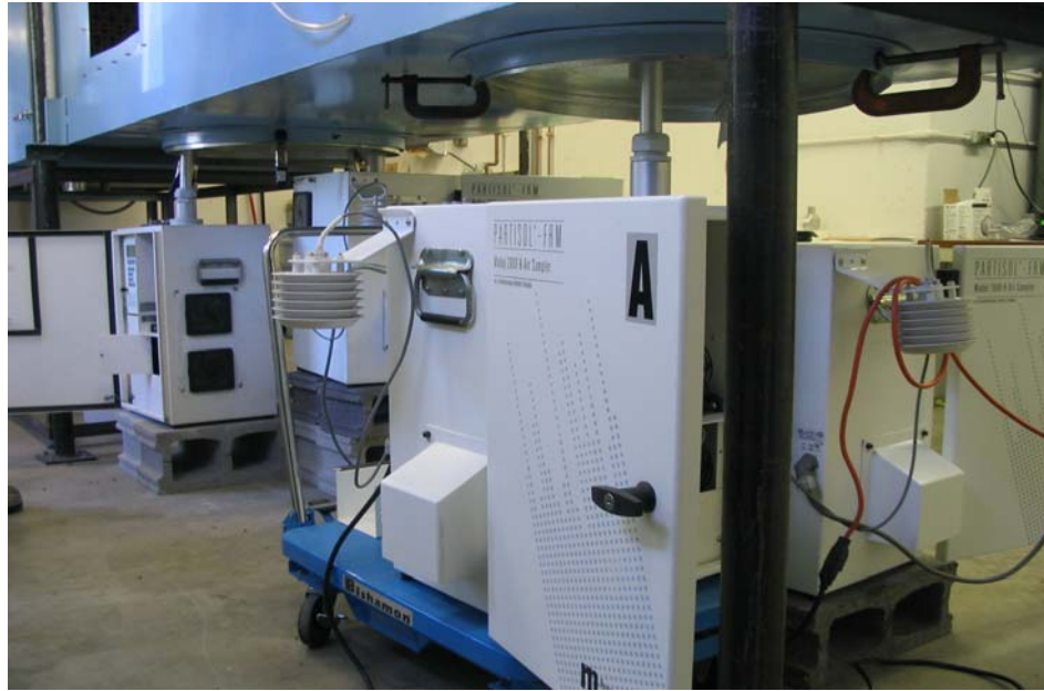
Figure 8. Partisol Sampler Bodies Below Exposure Section of Wind Tunnel
