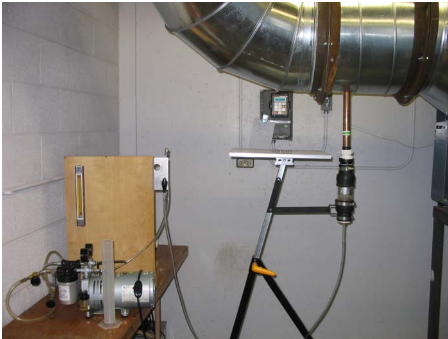
Figure 4. Fluidization System for Injecting Fine Fraction Dust Into the Flow System
