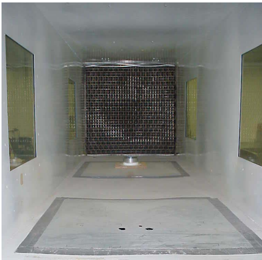
Figure 5. Test Chamber Interior With Flow Straightener (Viewed from downstream end of exposure section)
