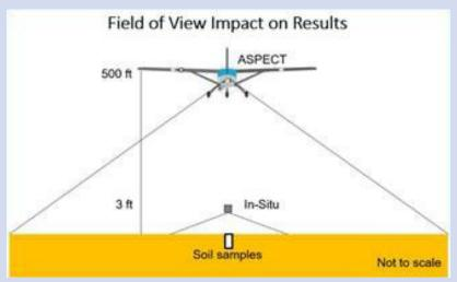
The ASPECT plane flies at around 300 feet above the ground, which gives it a field of view of approximately 6.5 acres. The data collected provides a general trend of areas containing elevated uranium or thorium levels. The exact area of contamination is further defined by ground surveys.
