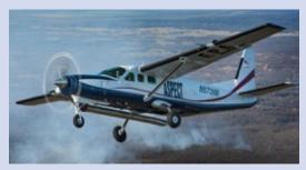
The ASPECT airplane is a cost-effective way to collect radiation data for large areas using state-of-the-art sensors to measure radiation levels on the ground.
