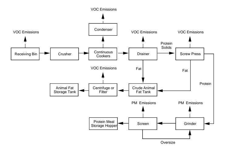
Figure 2-3. Continuous rendering process.
