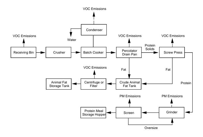
Figure 2-2. Batch cooker rendering process.
