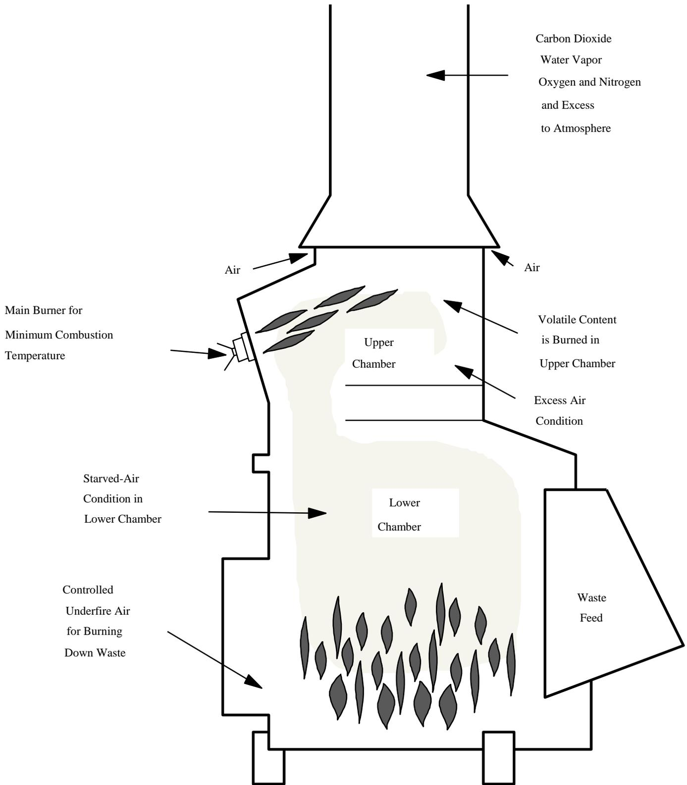
chamber heat release rates. Heat release rates for controlled air incinerators typically range from about 430,000 to 710,000 kJ/hr-m<sup>3</sup> (15,000 to 25,000 Btu/hr-ft<sup>3</sup>).
