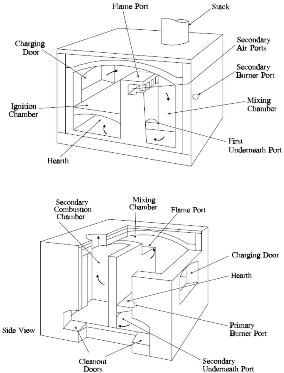
Figure 2.3-2. Excess Air Incinerator
