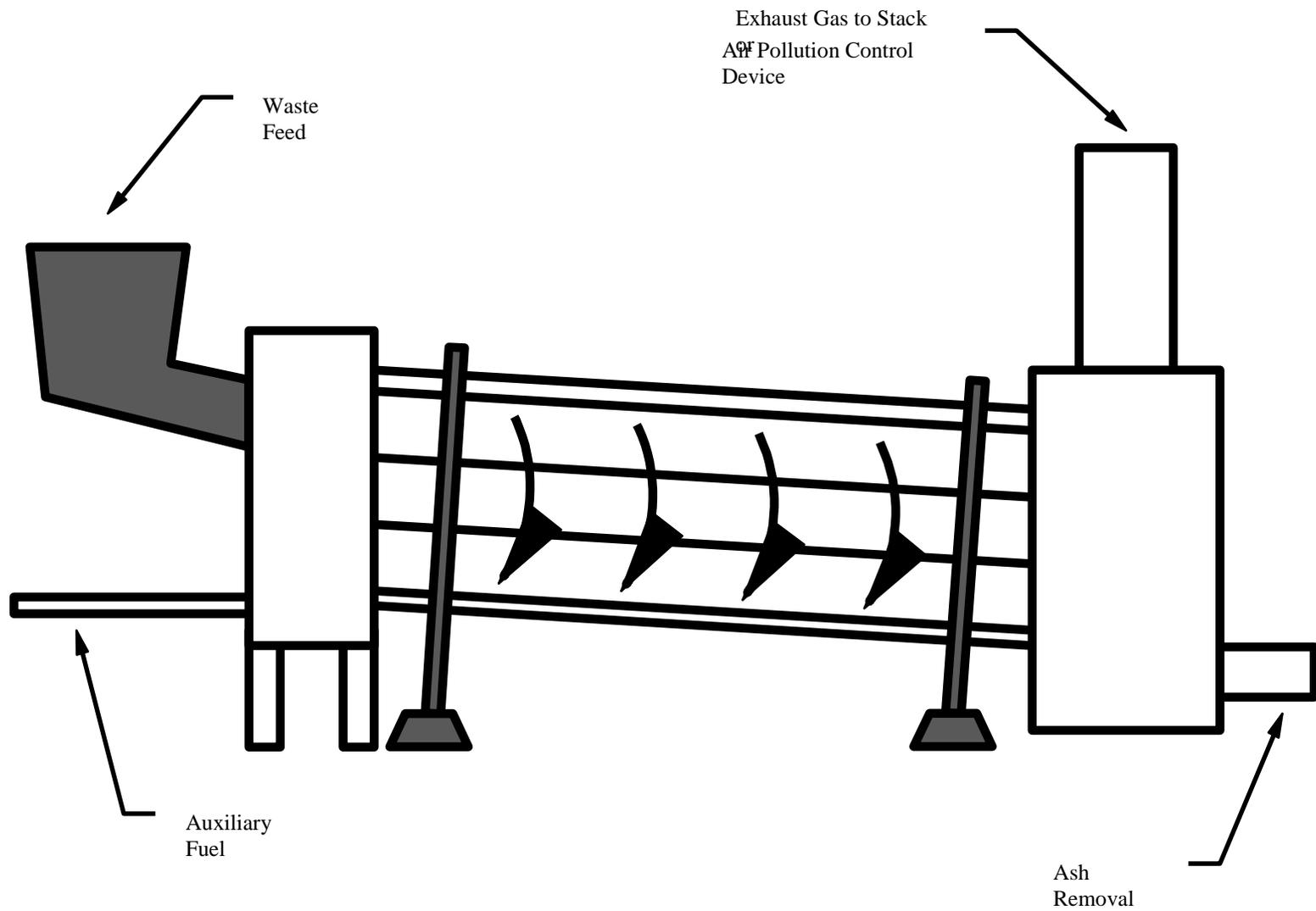
Figure 2.3-3. Rotary Kiln Incinerator
