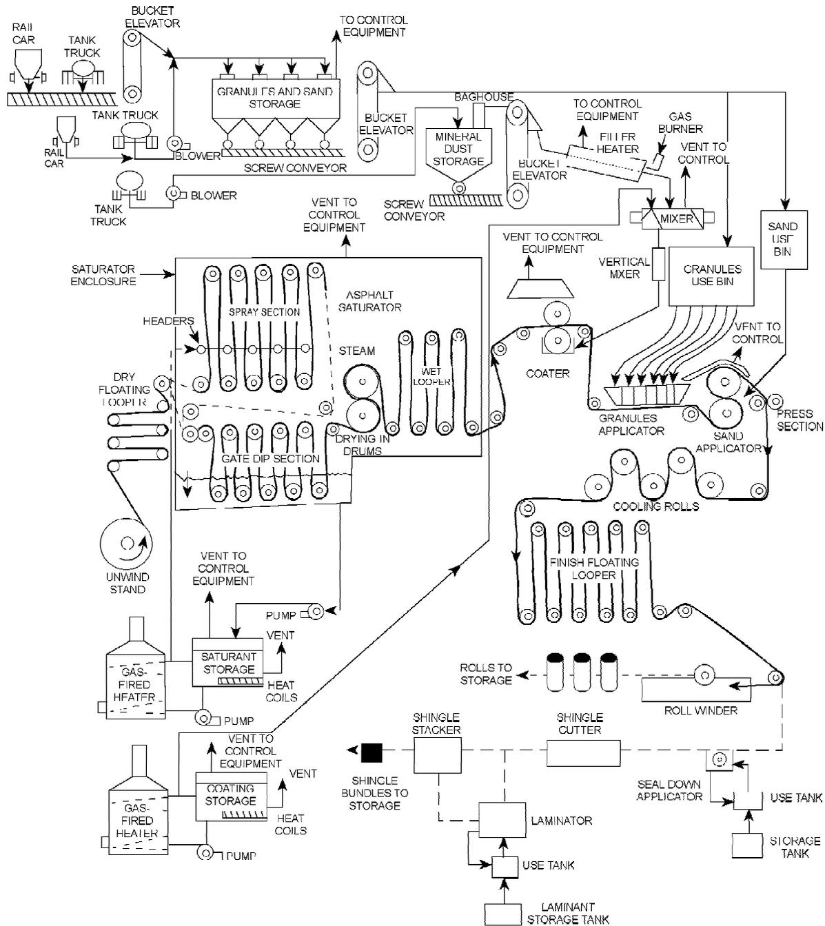
Figure 11.2-3. Organic shingle and roll manufacturing process flow diagram.<sup>1,2</sup>
