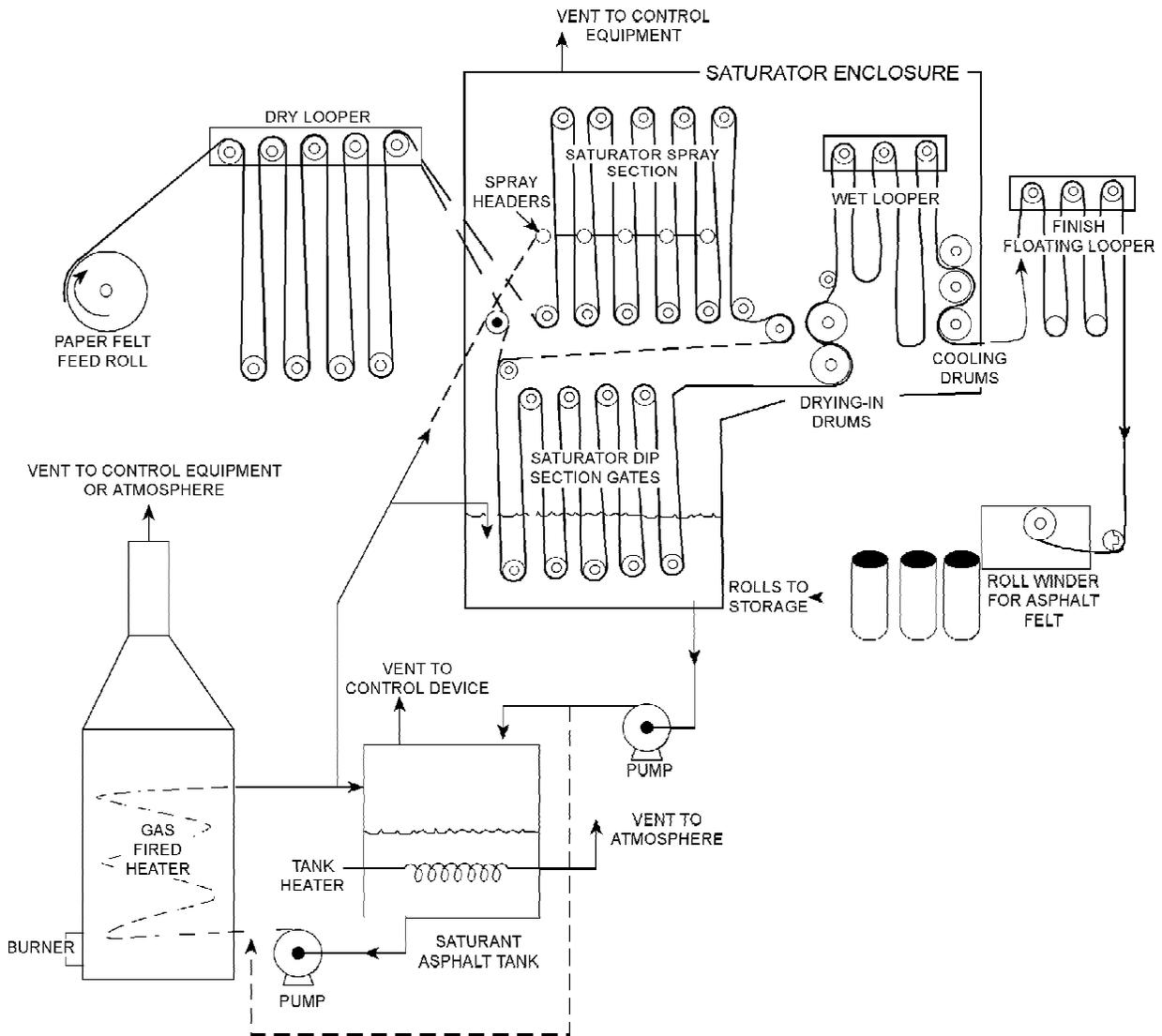
Figure 11.2-2. Asphalt-saturated felt manufacturing process.<sup>1,2</sup>
