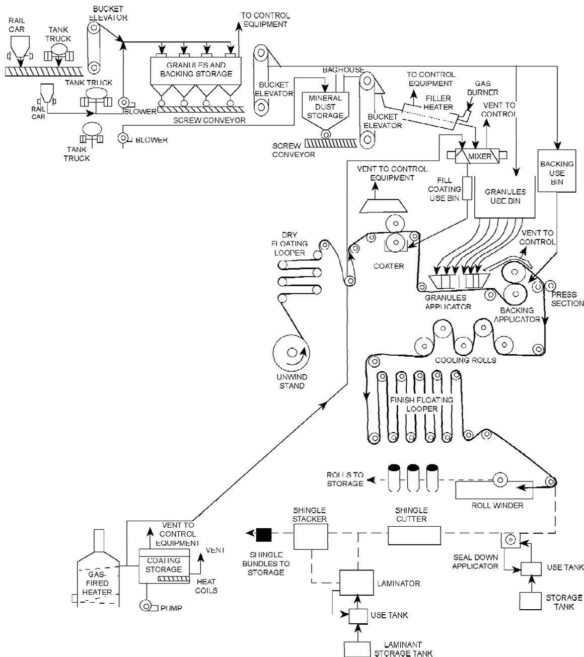
Figure 11.2-4. Fiberglass shingle and roll manufacturing process flow diagram.<sup>1,2</sup>
