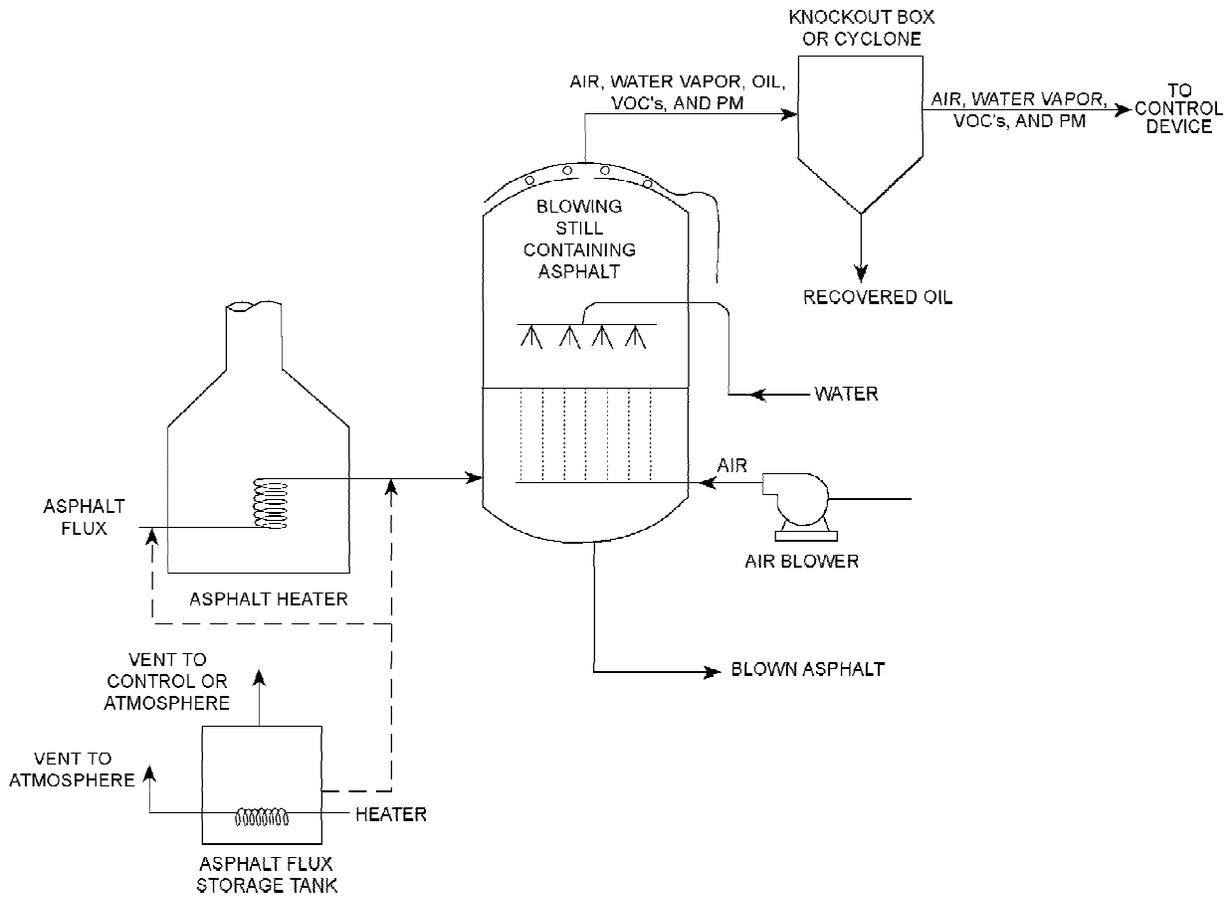
Figure 11.2-1. Asphalt blowing process flow diagram.<sup>1,4</sup>
