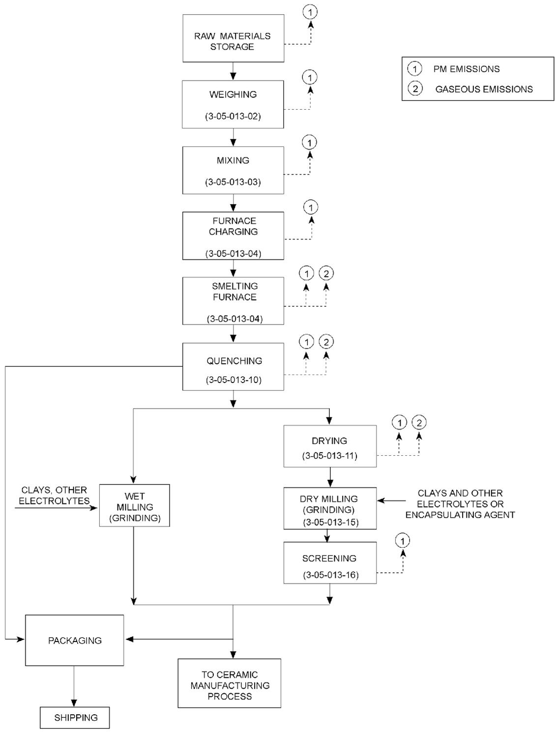
Figure 11.14-1 Process flow diagram for frit manufacturing.
