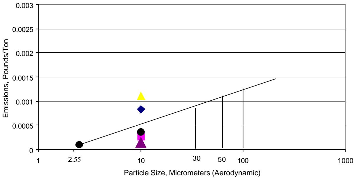
Figure 11.19-4. PM Emission Factor Calculation, Tertiary Crushing (Controlled)
