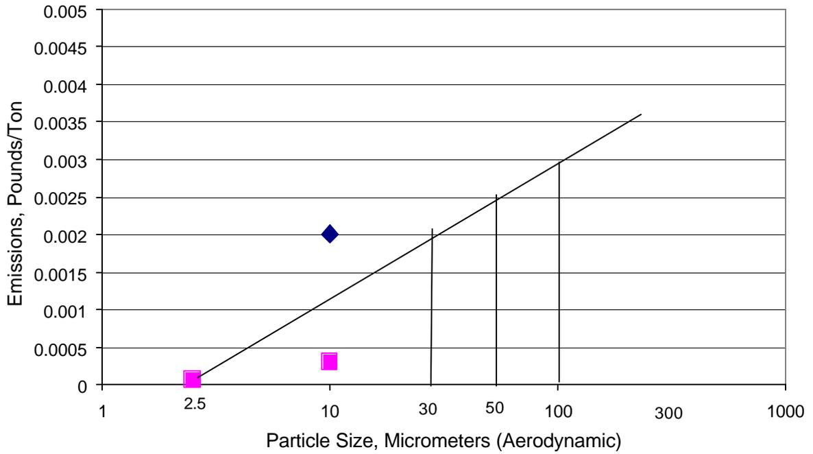
Figure 11-19.5. PM Emission Factor Calculation, Fines Crushing (Controlled)
