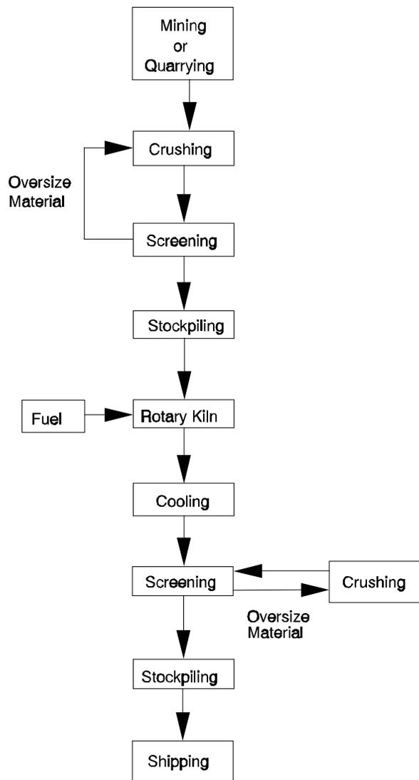
Figure 11.20-1. Process flow diagram for lightweight aggregate manufacturing.
