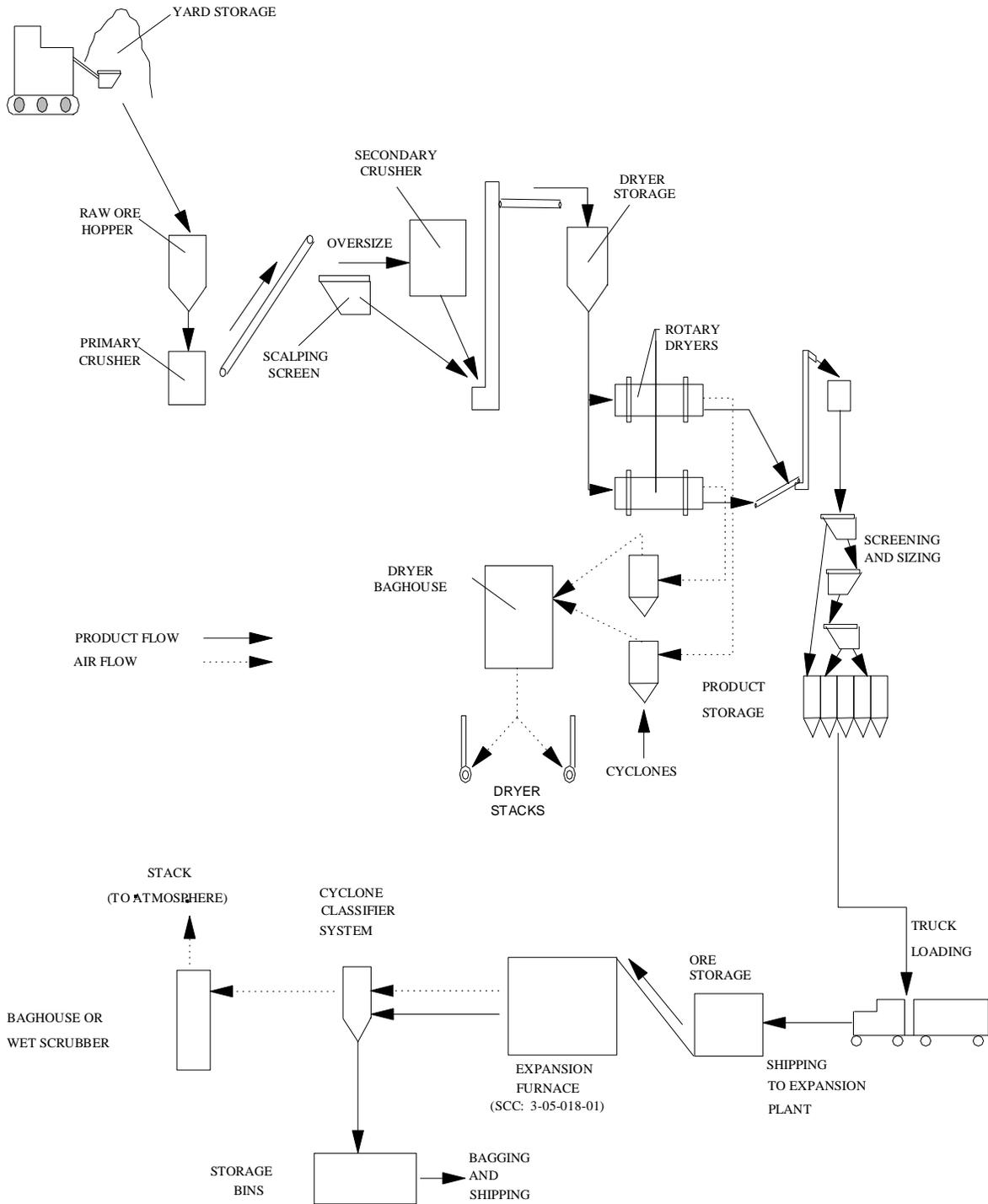
Figure 11.30-1. Flow diagram for perlite processing.<sup>1</sup>
