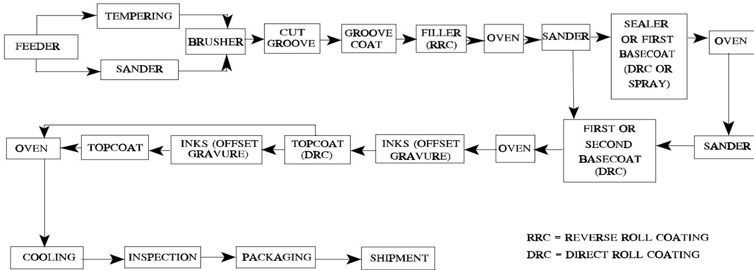
Figure 4.2.2.5-1. Flat wood interior panel coating line emission points.
