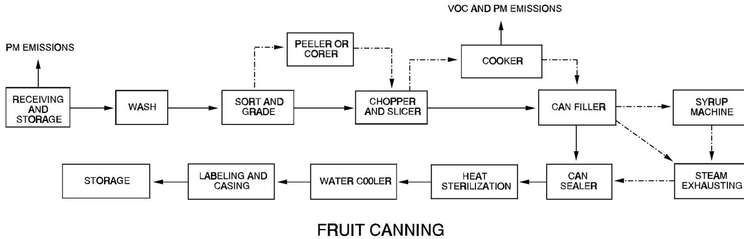
Figure 9.8.1-1. Generic process diagram for fruit canning.
