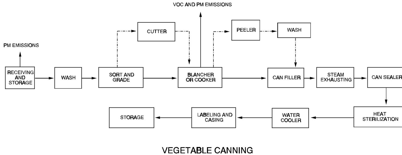
Figure 9.8.1-2. Generic process diagram for vegetable canning.
