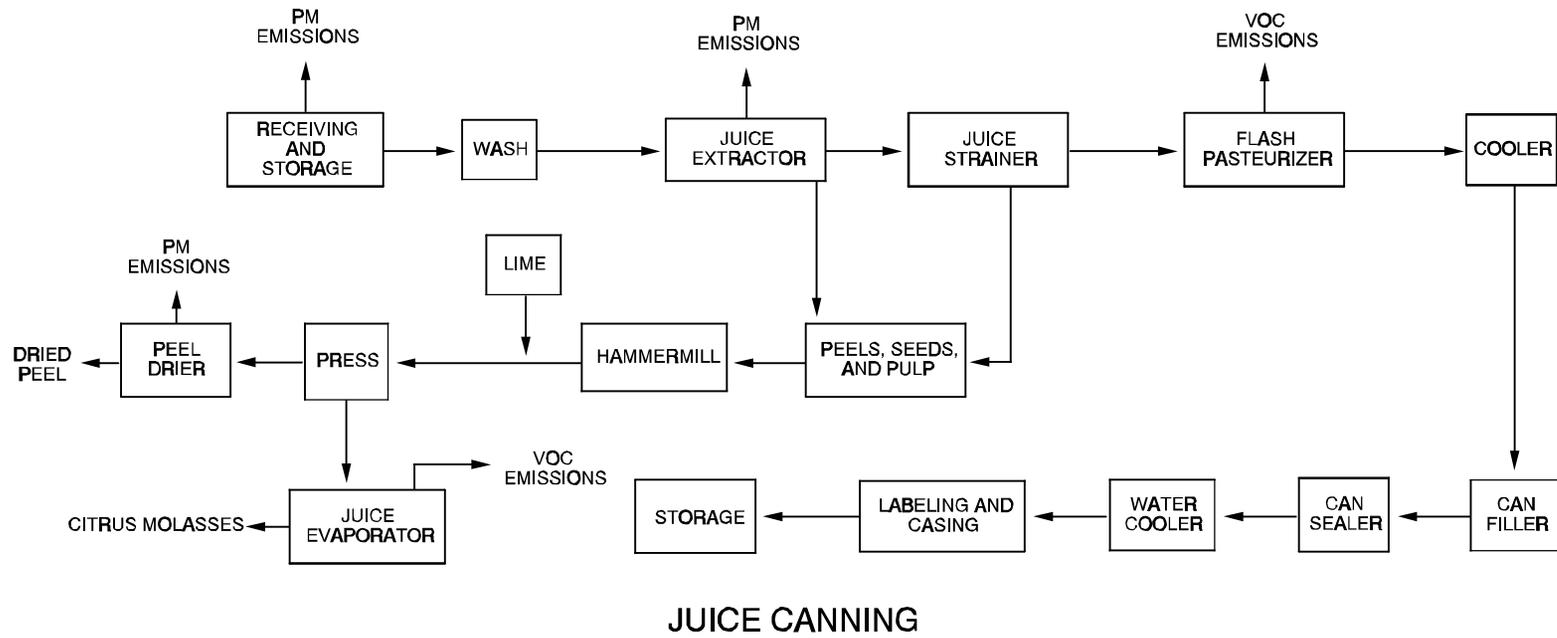
Figure 9.8.1-3. Generic process diagram for juice canning.
