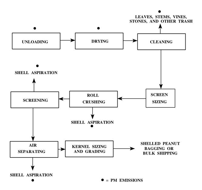
Figure 9.10.2.2-2. Typical shelled peanut processing flow diagram.
