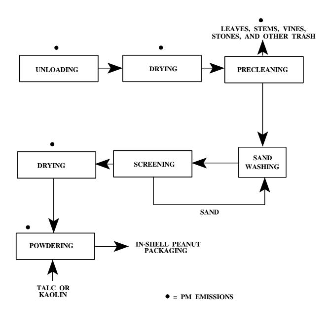
Figure 9.10.2.2-1. Typical in-shell peanut processing flow diagram.
