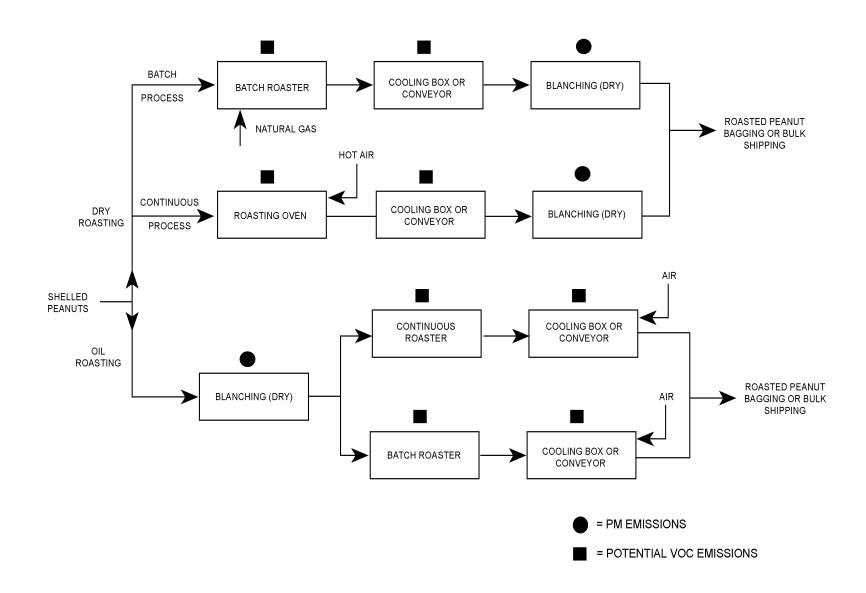
Figure 9.10.2.2-3. Typical shelled peanut roasting processing flow diagram.
