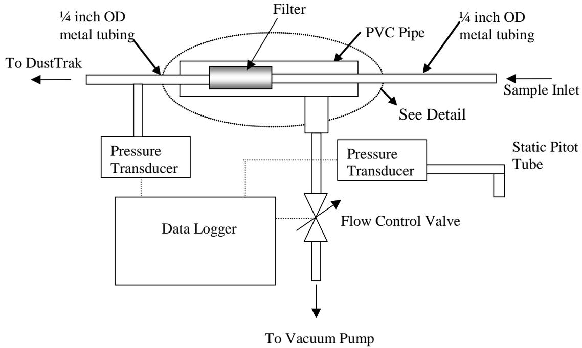
**Detail of Flow Splitting Section**
