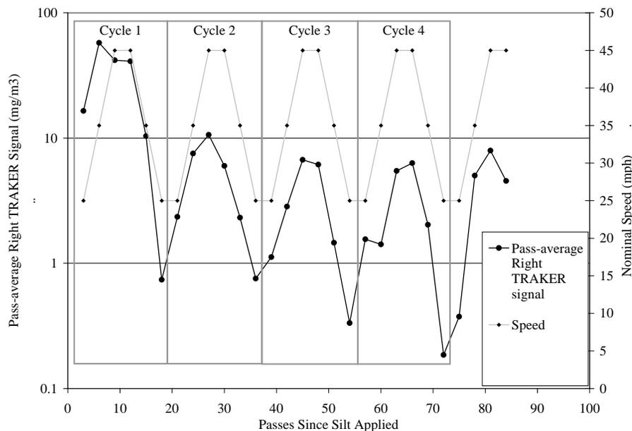
**Figure 5-11. Speed Response of TRAKER I Signal.** Figure shows the TRAKER I signal at each speed normalized to the average signal at 25 mph in the same cycle. Data are shown for 4 consecutive cycles as well as the average value for all cycles.
