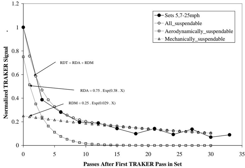
**Figure 5-9. Normalized TRAKER I Decay Curve for Sets 4, 6, and 8 (45 mph measurement) and Hypothesized Aerodynamically Suspending, Mechanically Suspending, and Total Suspending (aerodynamic plus mechanical) Road Dust Decay Curves**
