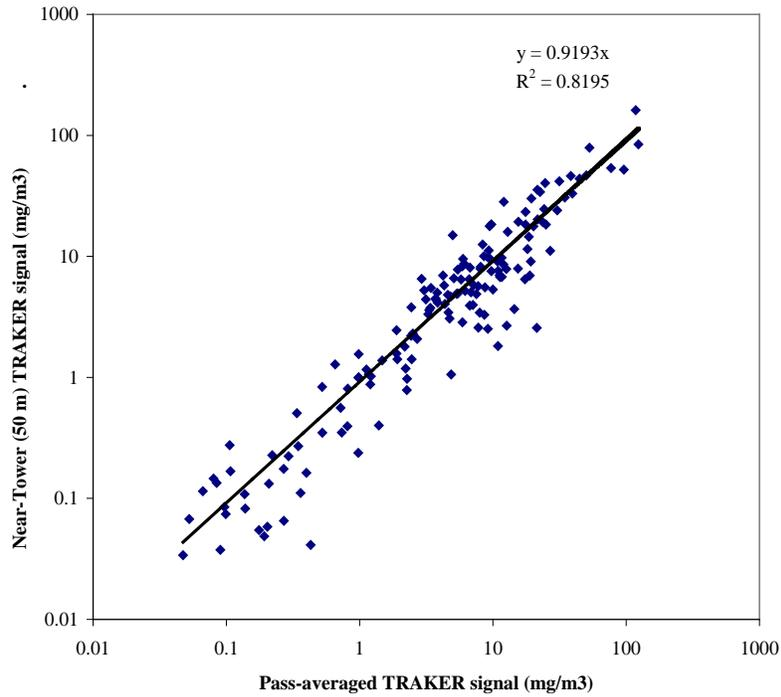
**Figure 5-4. TRAKER Signal (left and right) Averaged Over Entire Pass (pass-avg.) and Averaged Over Only the Portion of Test Road in the Vicinity of Flux Tower (Tower-avg.)**
