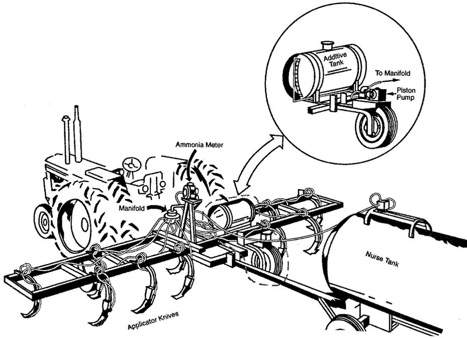
Figure 9.2.1-1. Typical trailer for application of anhydrous ammonia and fluid fertilizers.
