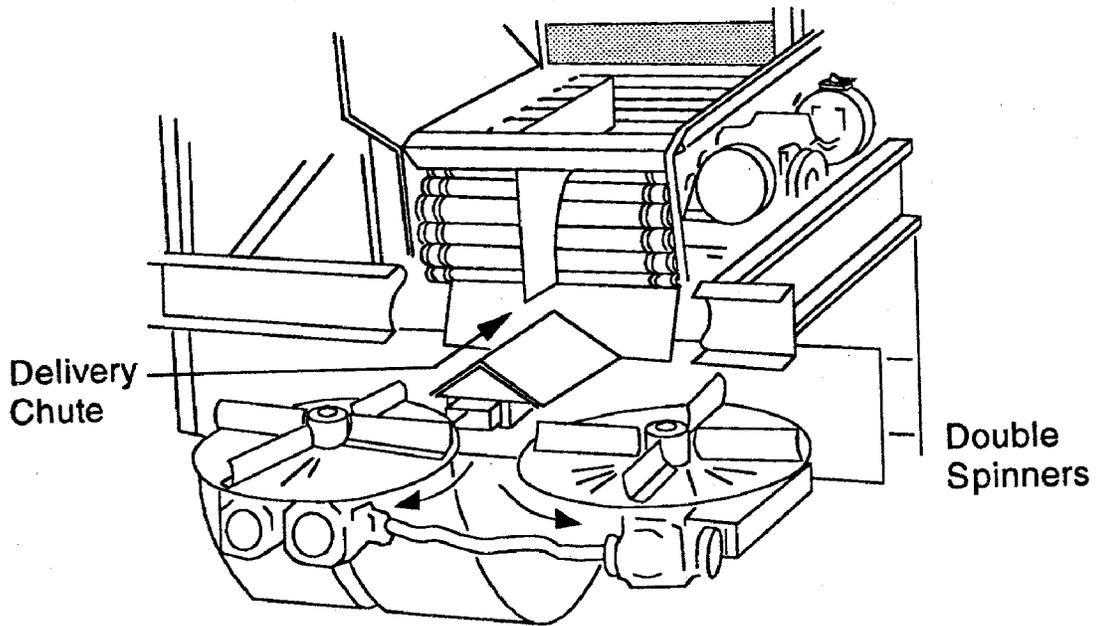
Figure 9.2.1-3. Example of centrifugal spreader.
