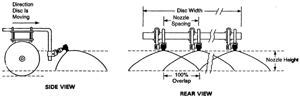
Figure 9.2.1-2. Side view and rear view of a typical spray nozzle system used for application of fluid fertilizers.
