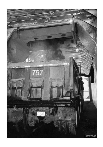
**Figure 6. Truck Loading Operations** with Fumes Being Captured by Hood
