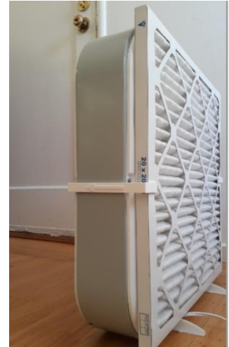
An example of a DIY air cleaner made with an air filter clamped onto a box fan.
