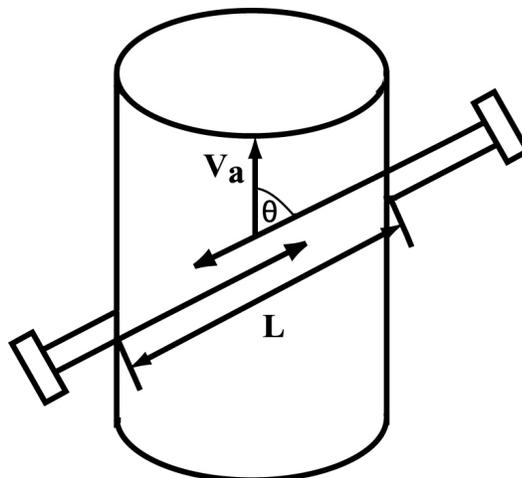
The velocity of the sound pulse through the stack gas is affected by the stack gas density, so changes in the stack temperature due to load changes, and/or temperature variations across the sonic path, will affect the flow measurement. In some cases correction factors can be developed using the pre-RATA testing to account for these changes.
