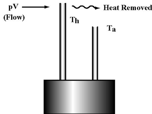
( $T_h$  = Temperature of Heated RTD,  $T_a$  = Temperature of Unheated RTD)
