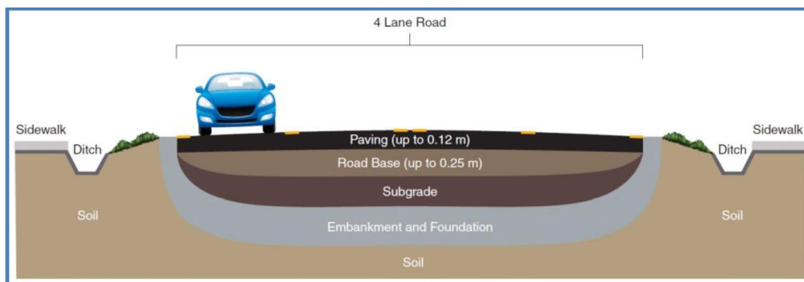
**Figure 4-1 Schematic Cross-Section of the Road Modeled by Arcadis 2019**
