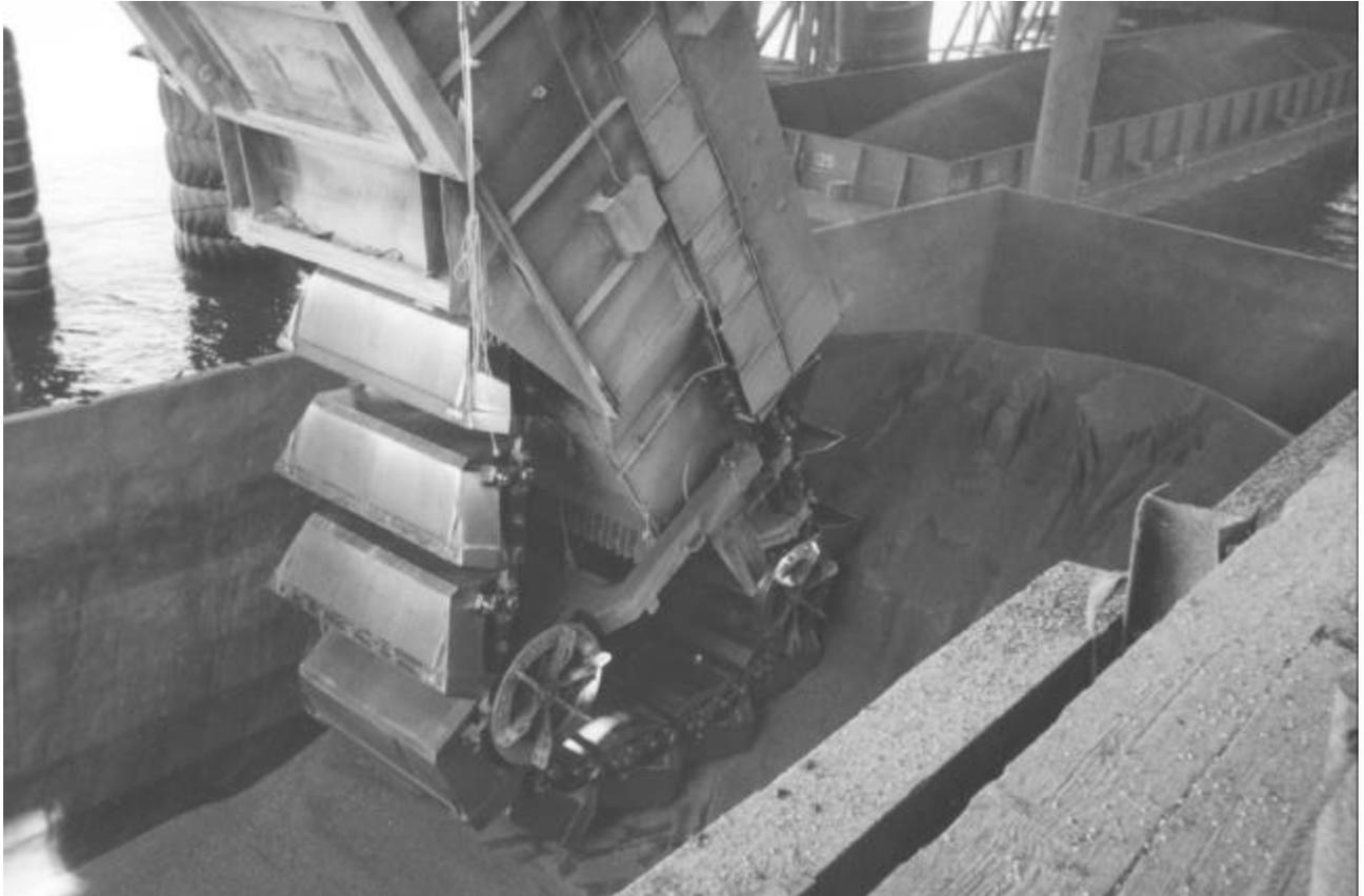
Photo 3. Marine leg barge unloader.
