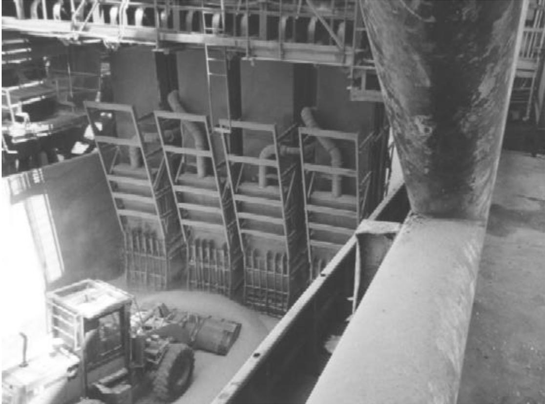
Photo 4. Straight vessel (ship) loading spout.
