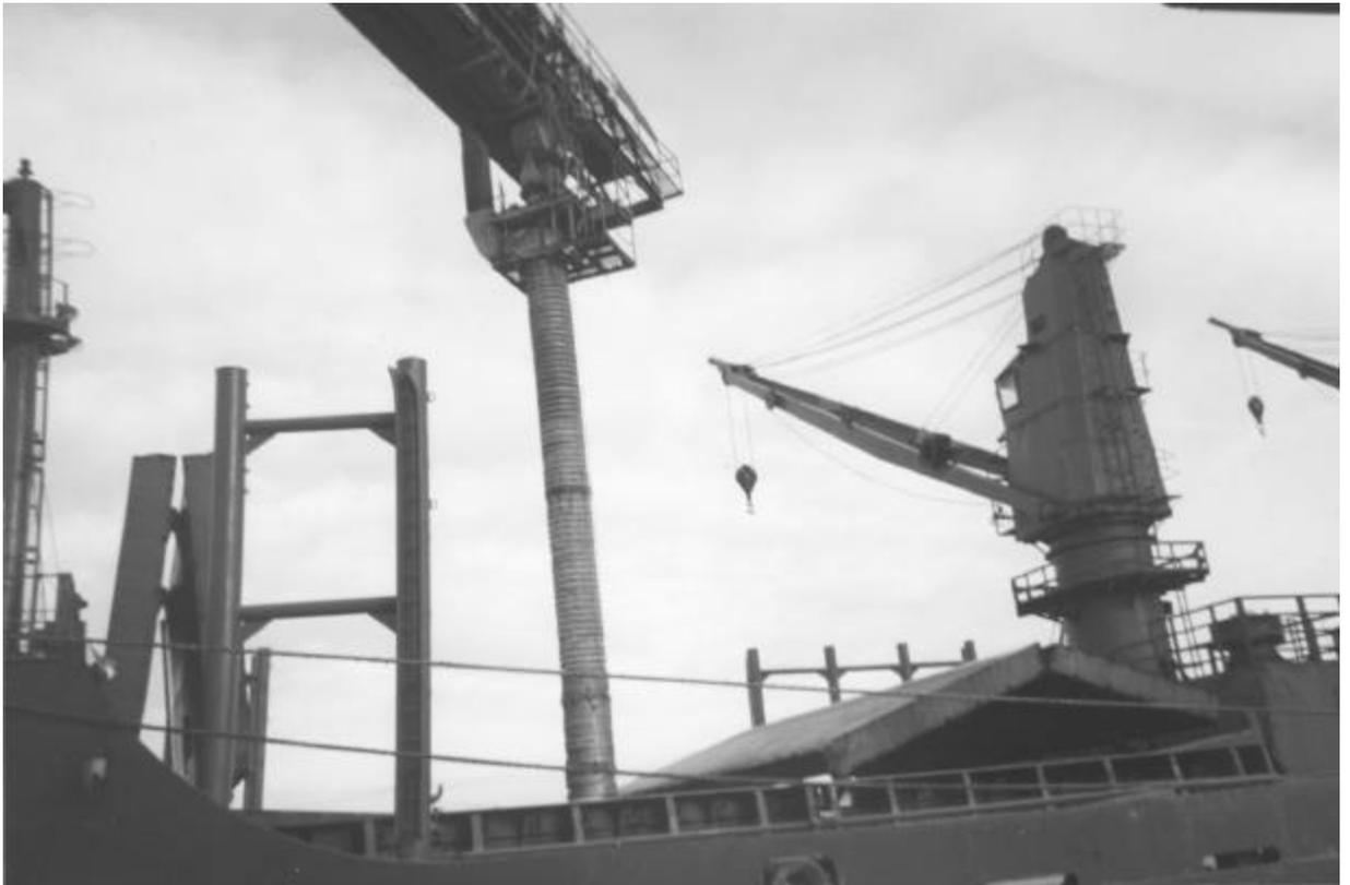
Photo 5. Sloped vessel (ship) loading spout.
