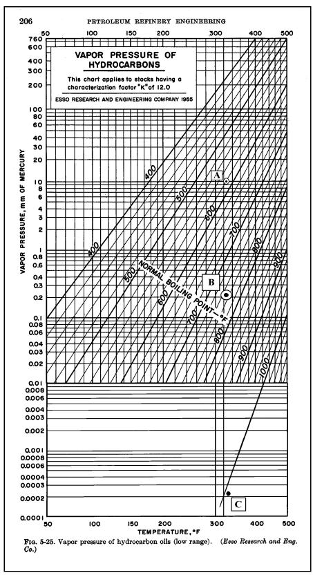
Figure 11. Vapor Pressure of Hydrocarbons. Adapted from Petroleum Refinery Engineering, W. L. Nelson, 1958.
