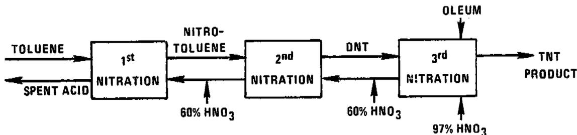
Figure 5.6-2. Nitration of toluene to form trinitrotoluene.
