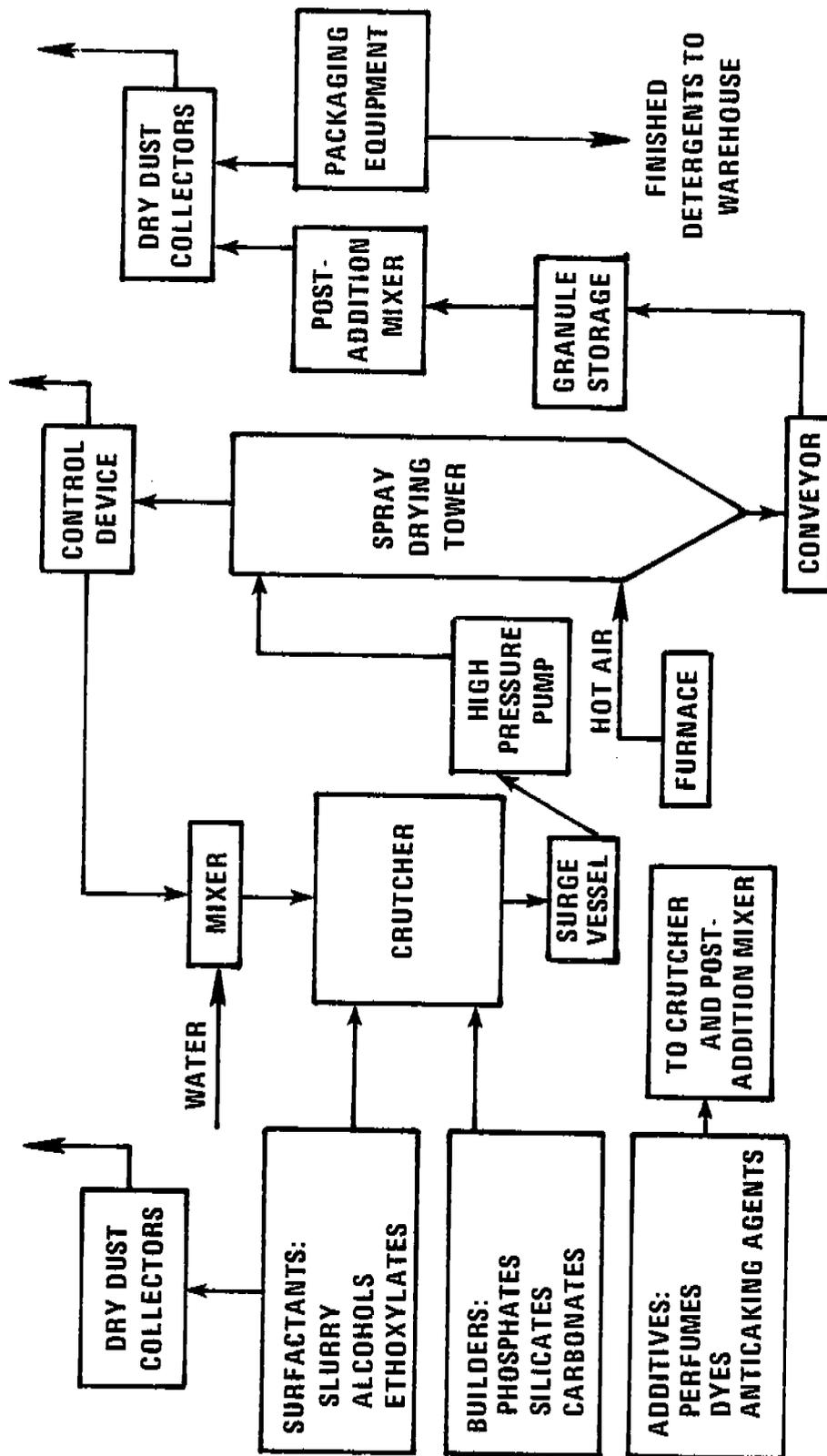
Figure 5.15-1. Manufacture of spray dried detergents.
