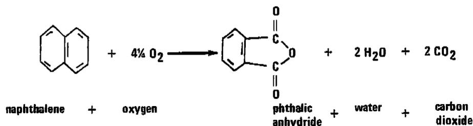
The reactor effluent containing crude PAN plus products from side reactions and excess oxygen passes to a series of switch condensers where the crude PAN cools and crystallizes. The condensers are alternately cooled and then heated, allowing PAN crystals to form and then melt from the condenser tube fins.
