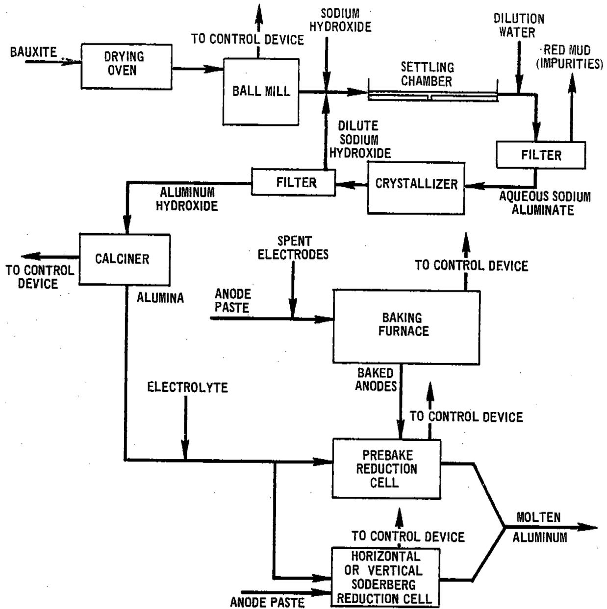
Figure 7.1-1. Schematic diagram of primary aluminum production process.
