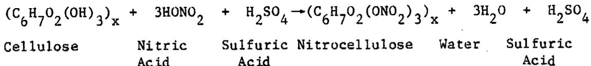
Following nitration, the crude NC is centrifuged to remove most of the spent nitrating acids and is put through a series of water washing and boiling treatments to purify the final product.
