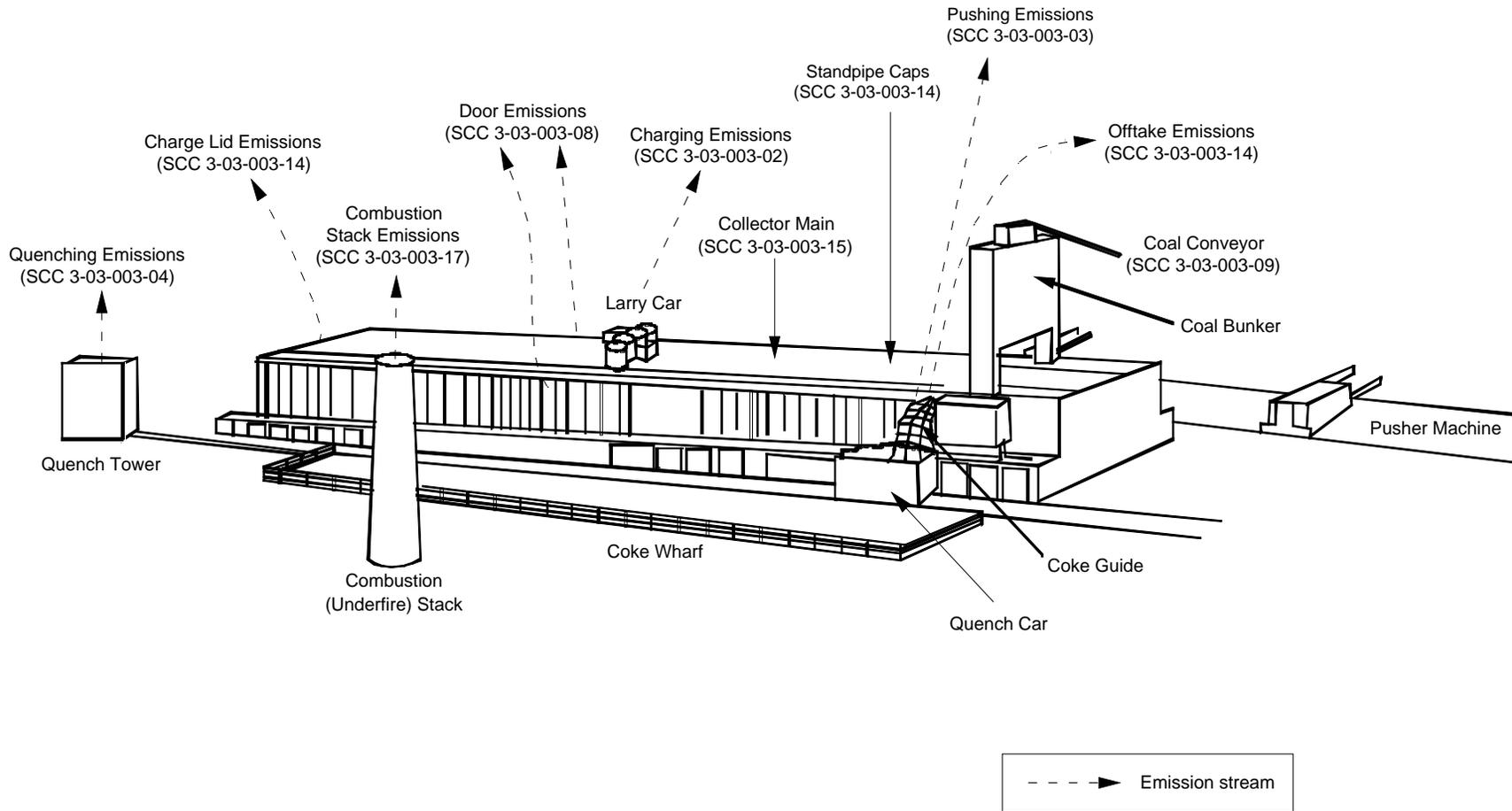
Figure 2-1. Byproduct coke oven battery showing major emission points.
