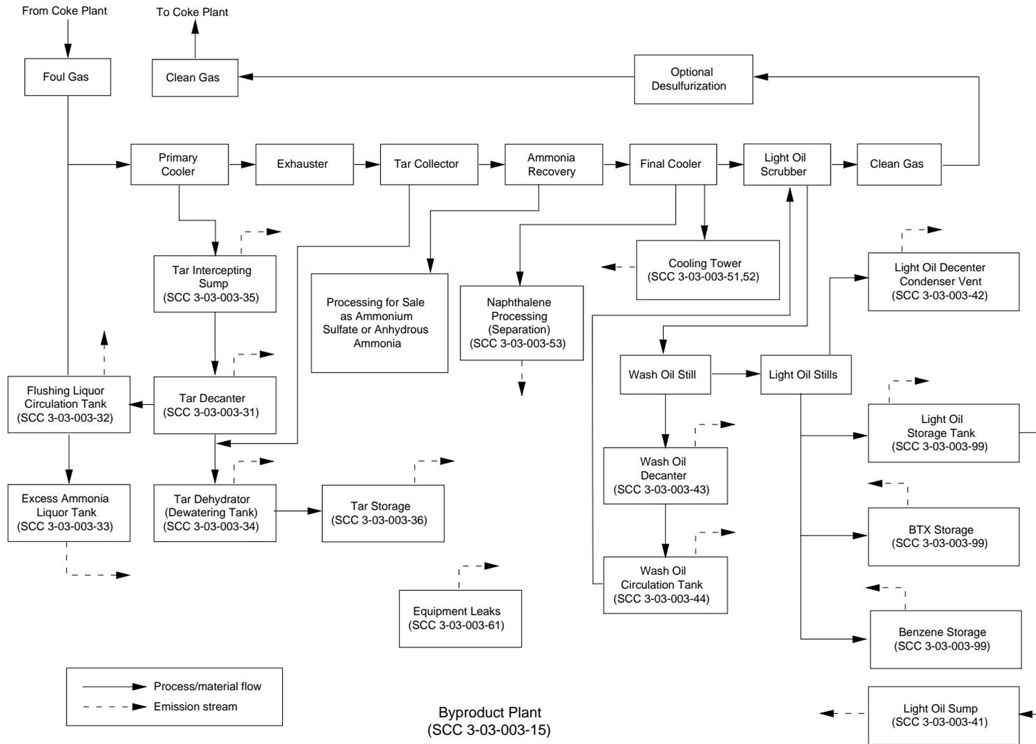
Figure 2-3. Flow diagram for coke byproduct recovery plant.
