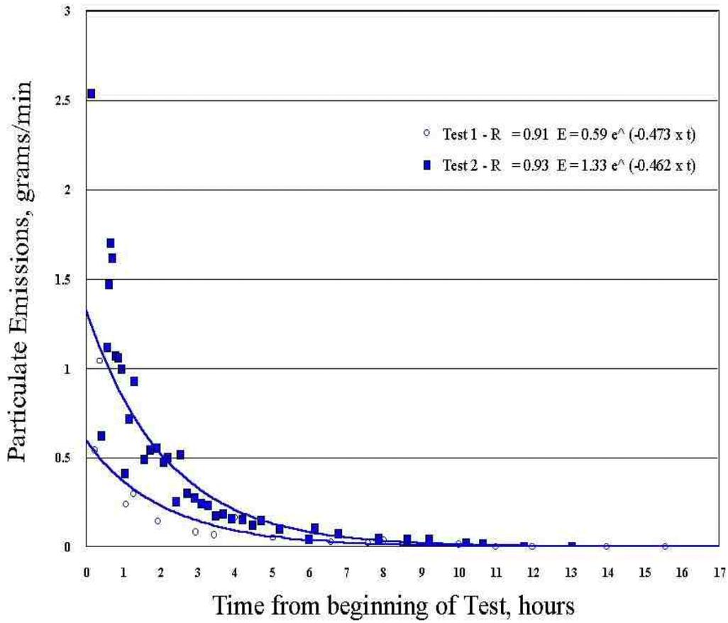
Figure 4-1. Coke oven door emissions versus time after charging from Reference 181.
