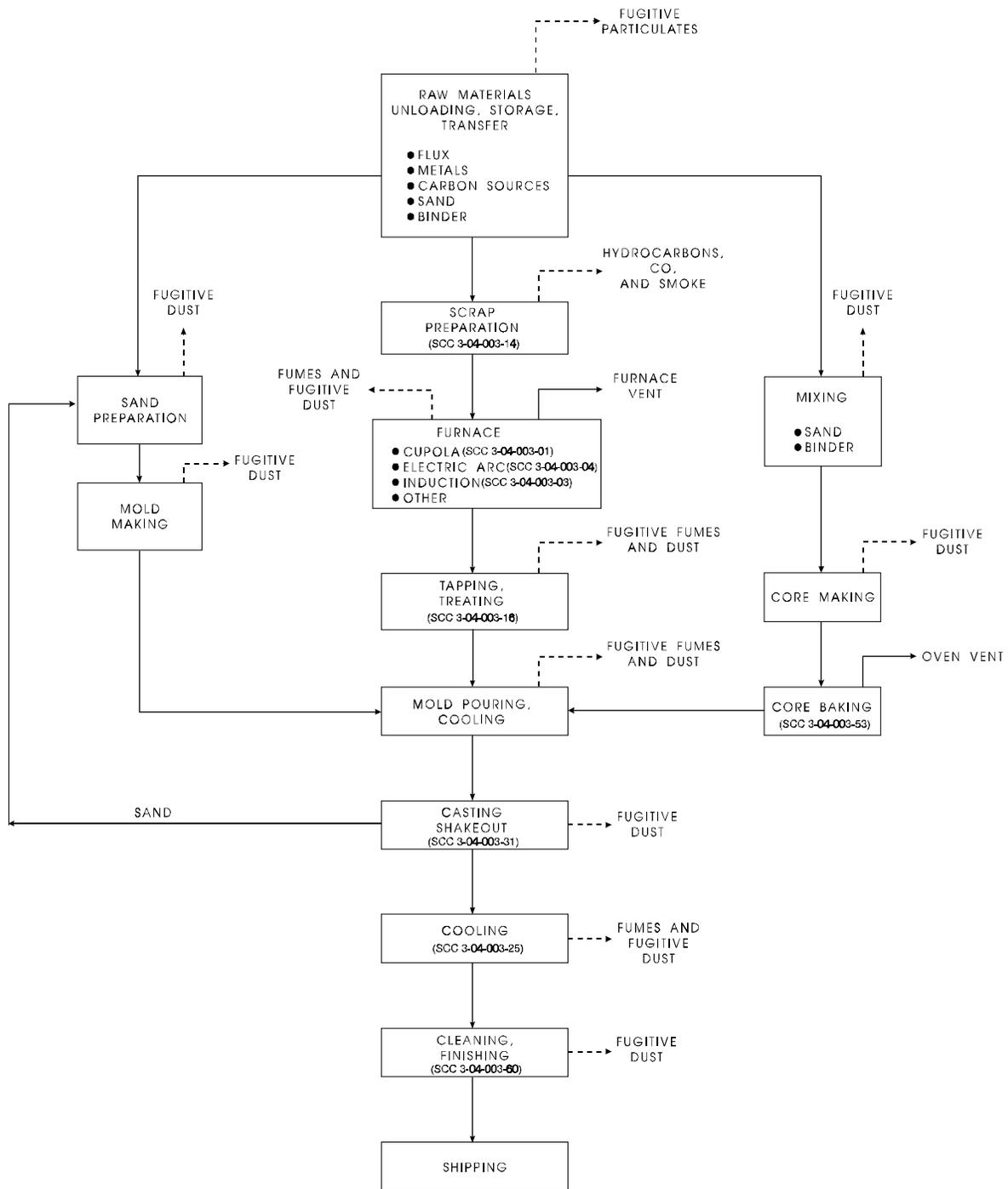
Figure 12.13-1. Flow diagram of a typical steel foundry.
