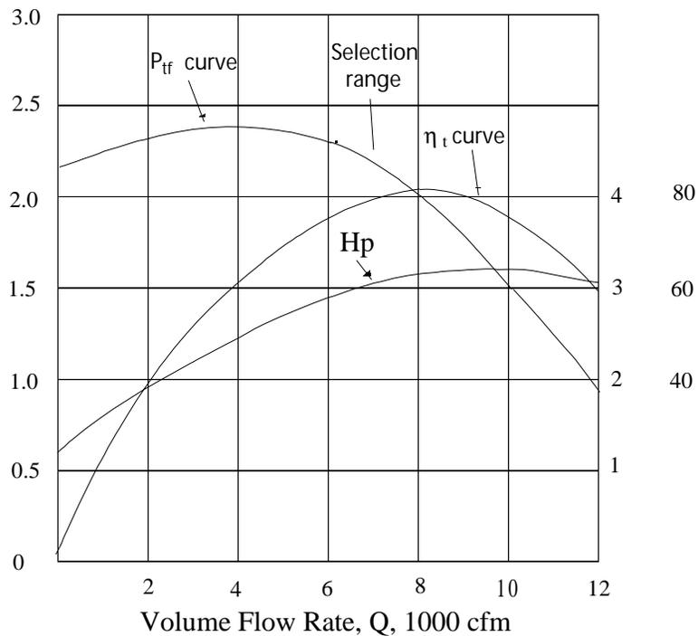
**Figure 3.6:** Conventional Fan Performance curve used by most manufactures
