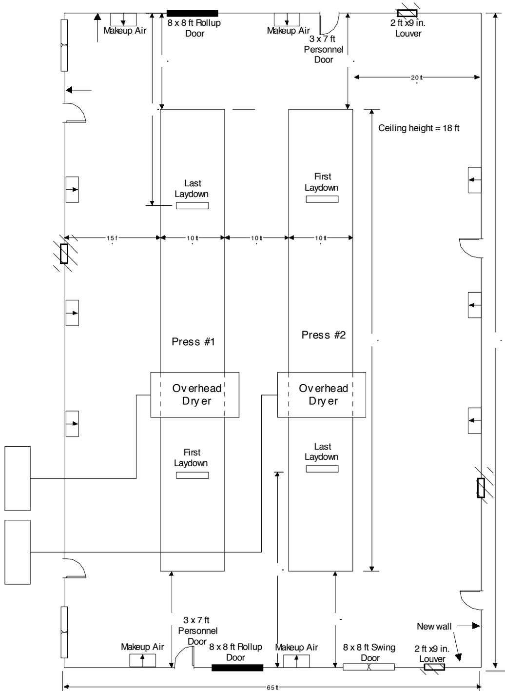
**Figure 3.8:** Example Permanent Total Enclosure
