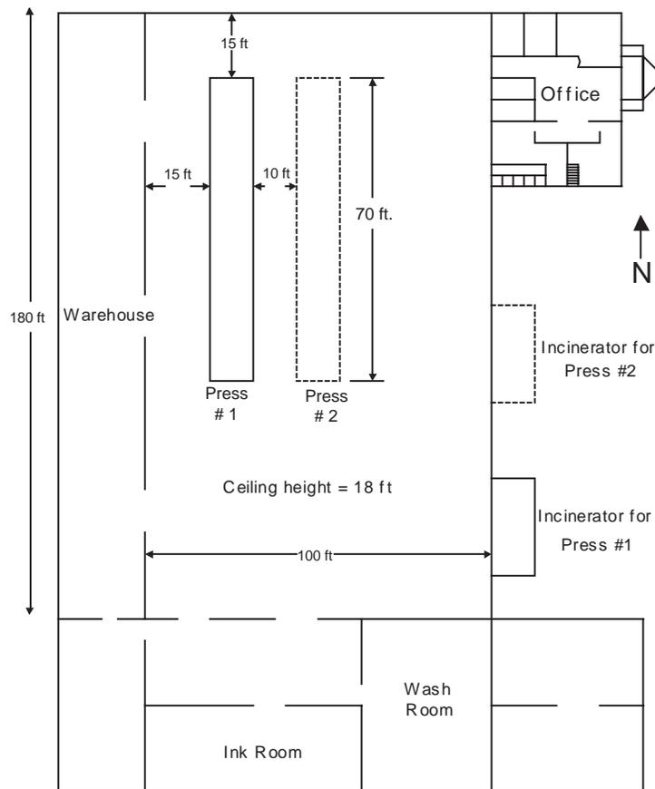
**Figure 3.7: Example Plant Layout**
