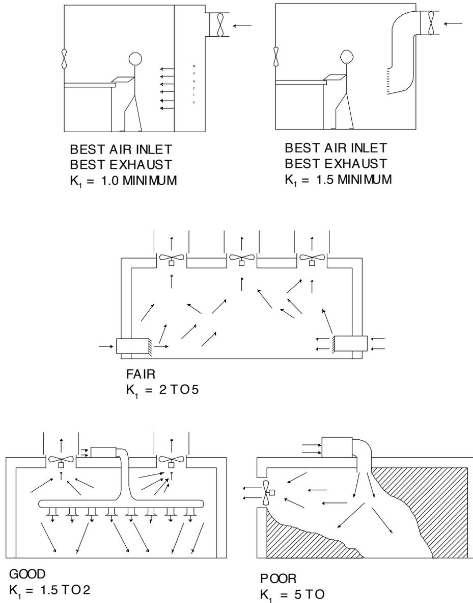
**Figure 3.1:** Typical  $K_1$  Factors Based on Inlet and Exhaust Locations
