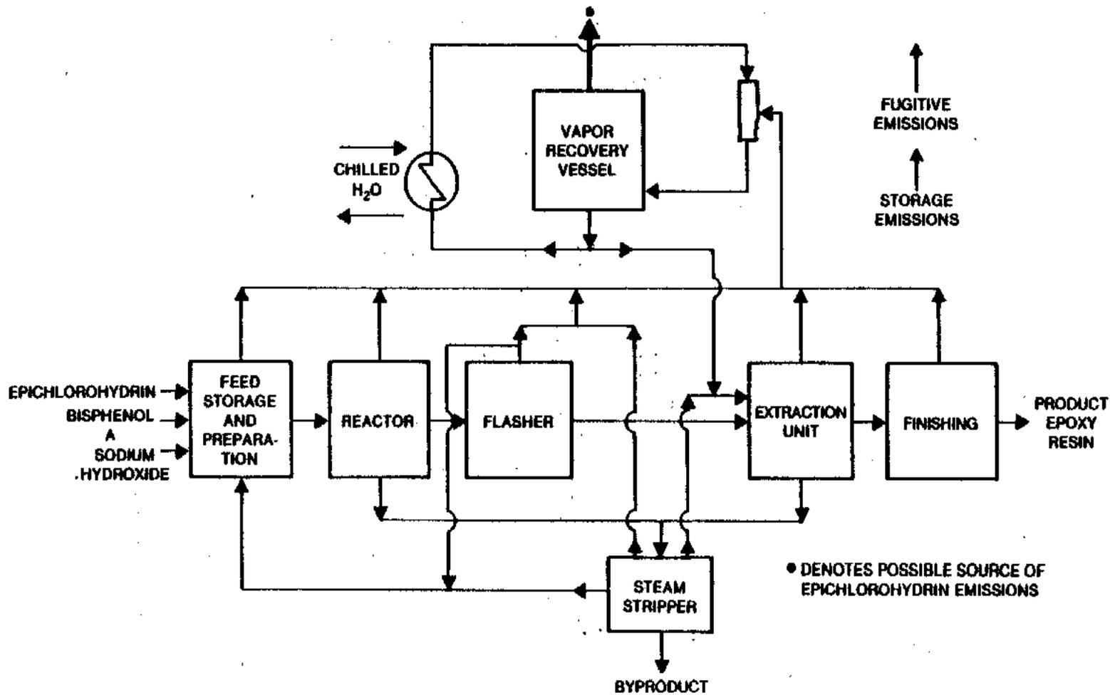
Figure 3. Basic operations that may be used in the continuous production of epoxy resins from epichlorohydrin (well-controlled facility).
