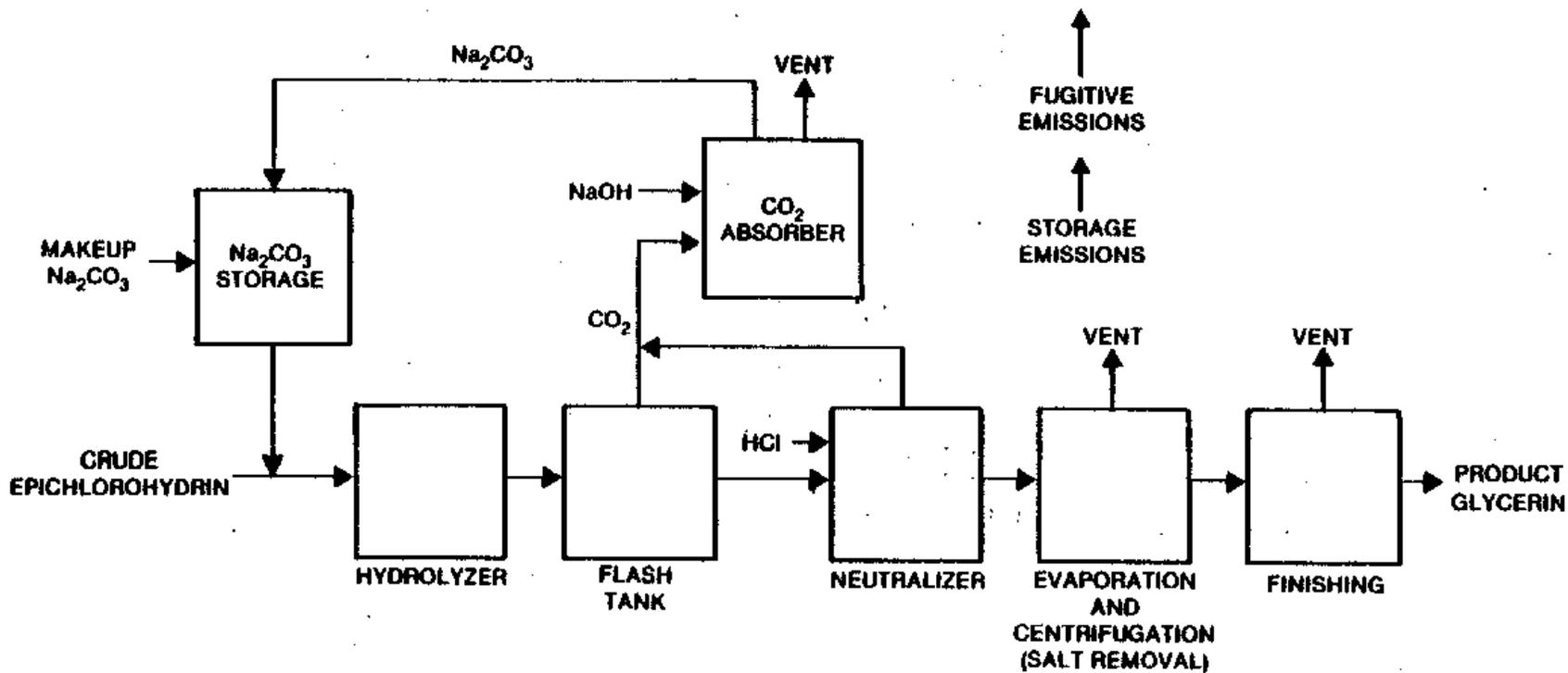
Figure 2. Basic operations that may be used in the production of synthetic glycerin from epichlorohydrin.
