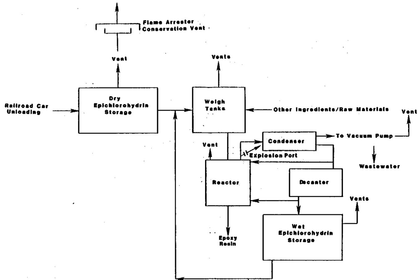
Figure 4. Flow diagram for the batch production of epoxy resins. <sup>11</sup>
