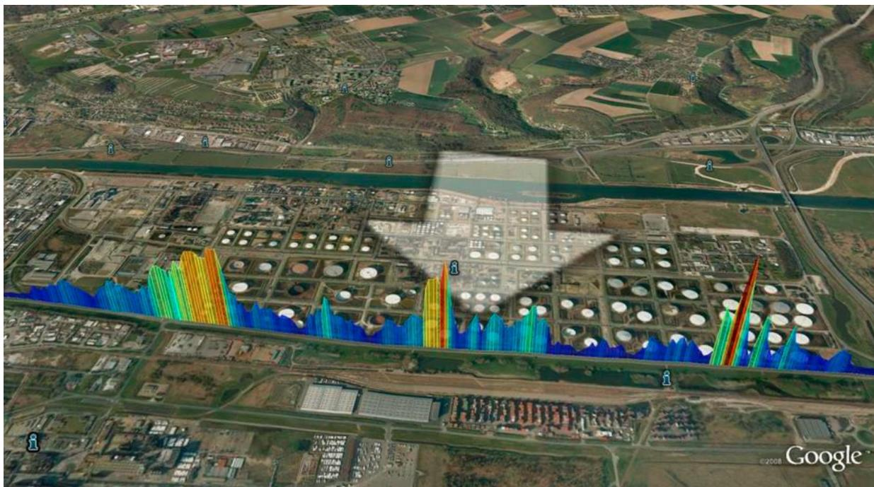
**Figure 3-3. Illustration of a SOF transect past a refinery (from Mellqvist et al., 2014a)**
