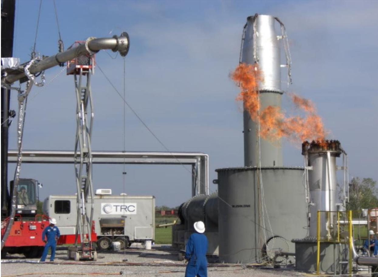
**Figure 3-4. Picture of extractive sampling system used as part of the 2010 TCEQ flare study project (from Allen and Torres, 2011)**
