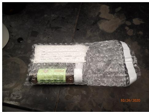
Description: Sample package for composite sample which is sent to Microbac Lab. Location: Environmental Laboratory. Date/Time: October 26, 2020 11:14 A.M.
