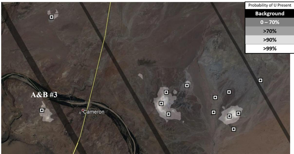
*Figure 87: Closer view of the Cameron area within Zone 3. This product is not correlated to concentration and should be used to identify areas where further ground-based characterization efforts may be warranted.*
