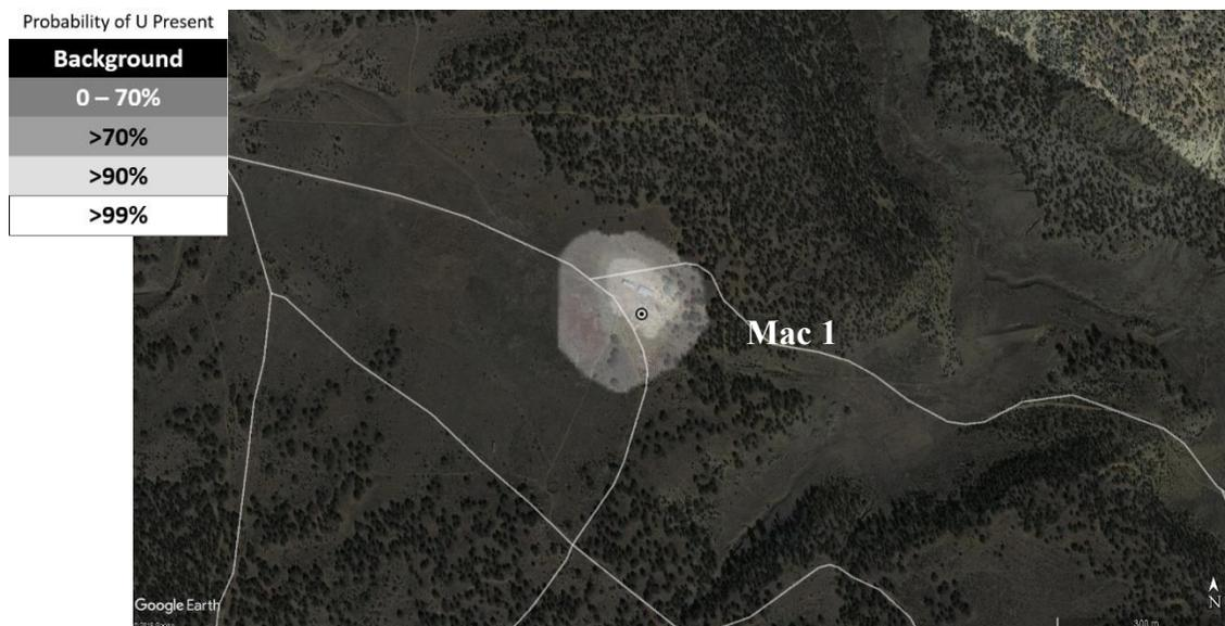
Figure 24: Close-up view of Mac 1 mine with the PUP product. Probability of Uranium Present (PUP) product shows areas where natural uranium is out of balance (white) with the natural background (black). White areas indicate where uranium spectral signatures are statistically significantly present for uranium and its decay products. **This product is not correlated to concentration and should only be used to identify areas where further ground-based characterization efforts may be warranted.**
