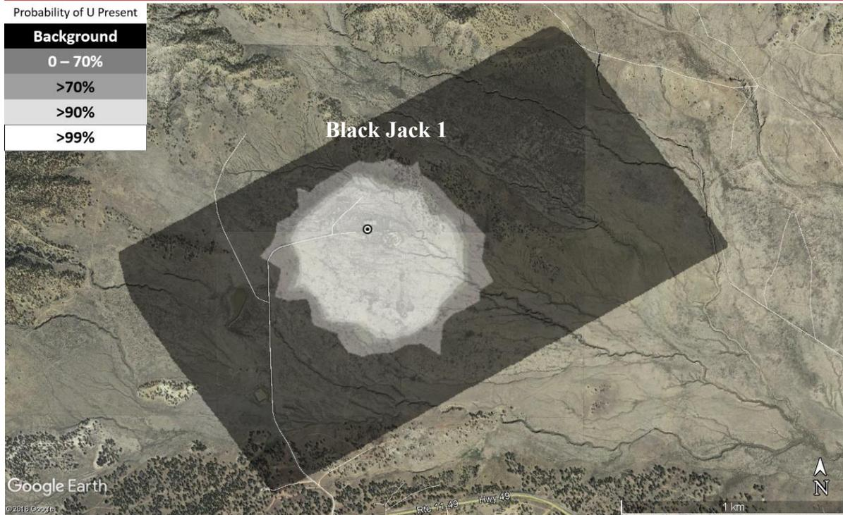
*Figure 10: Probability of Uranium Present (PUP) product shows areas where natural uranium is out of balance (white) with the natural background (black). White areas indicate where uranium spectral signatures are statistically significantly present for uranium and its decay products. This product is not correlated to concentration and should only be used to identify areas where further ground-based characterization efforts may be warranted.*
