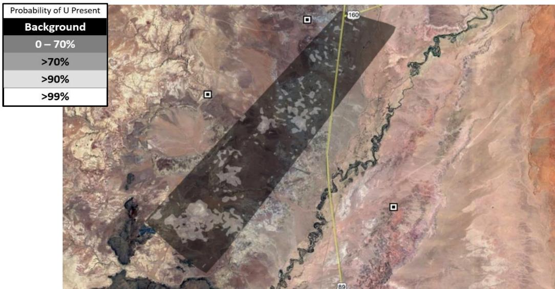
Figure 103: The PUP product shows areas where natural uranium is out of balance (white) with the natural background (black). White areas indicate where uranium spectral signatures are statistically significantly present for uranium and its decay products. There appears to be several areas with natural uranium outcropping. **This product is not correlated to concentration and should be used to identify areas where further ground-based characterization efforts may be warranted.**
