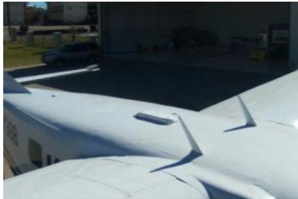
*Figure 111: ASPECT satellite communication system phased array antenna.*
