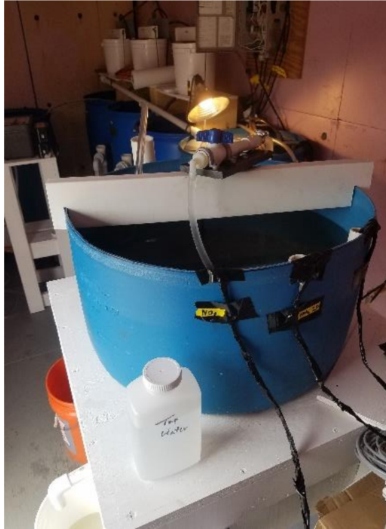
Testing to develop a low-cost sensor to record nitrogen concentration in effluent released from innovative/alternative septic systems. Location: Massachusetts Alternative Septic System Test Center
