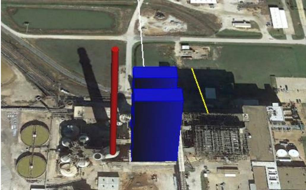
**Figure 2-8. A Satellite View of the Pirkey Power Plant in November 2013 Illustrating the Shadow Length for the Stack (173 m), the Adjacent Building (29 m), and the Second Building (89 m), Located Further Away to the Right.**
