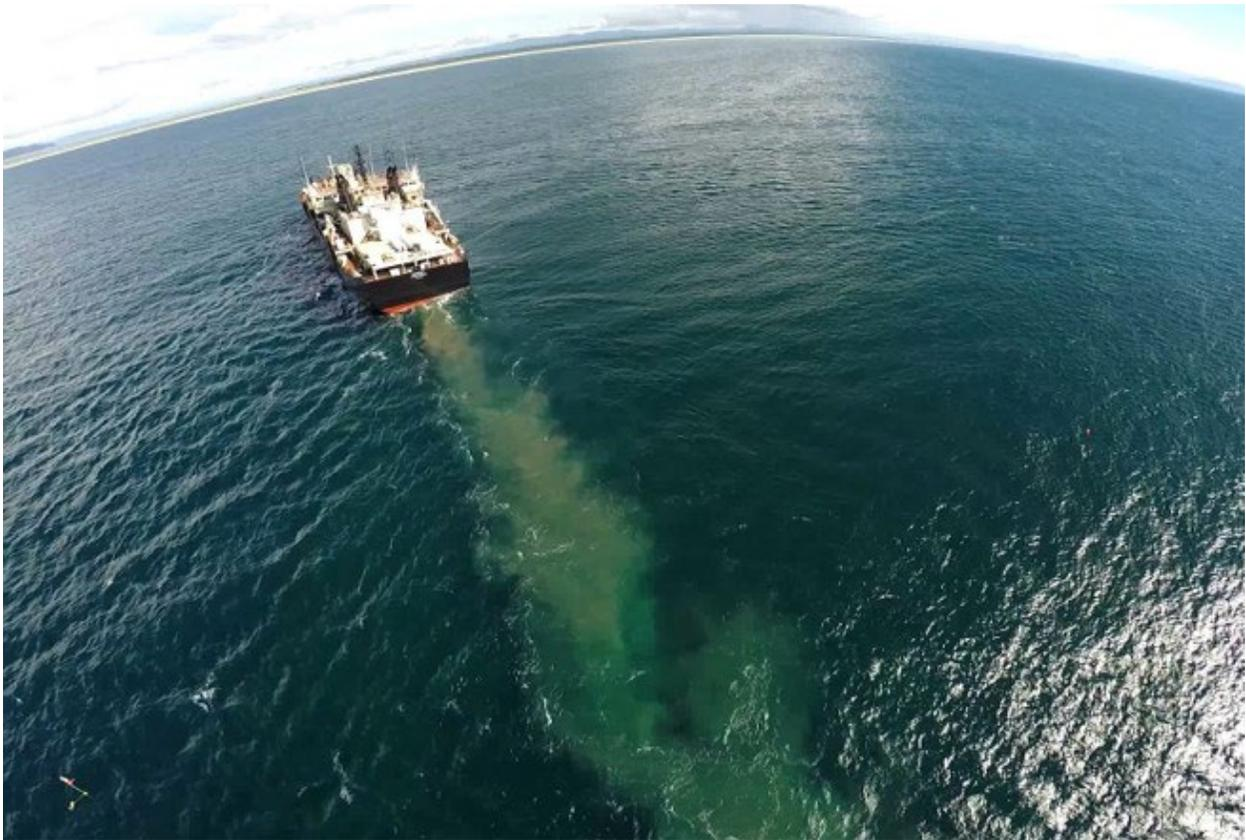
**Figure 25.** Aerial view of the *Essayons* during nearshore thin-layer sand placement operations near the mouth of the Columbia River. The disposal vessel moves forward slowly with hull doors only partially opened, so that sand is spread thinly in long, narrow tracks. The ship’s propellers help to further disburse the sand.
