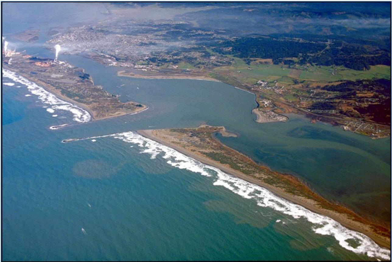
**Figure 21.** Looking northeast toward the Humboldt Entrance Channel and Jetties. Note the spits with beaches and extensive dune systems to the north and south of the Entrance Channel (photograph by Gary Todoroff).
