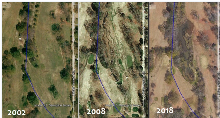
Figure 3. Changes can be seen by comparing the project area in 2002 (left, before restoration), 2008 (middle, after stream restoration), and 2018 (right, after a beaver dam impoundment formed in the restored stream channel).
