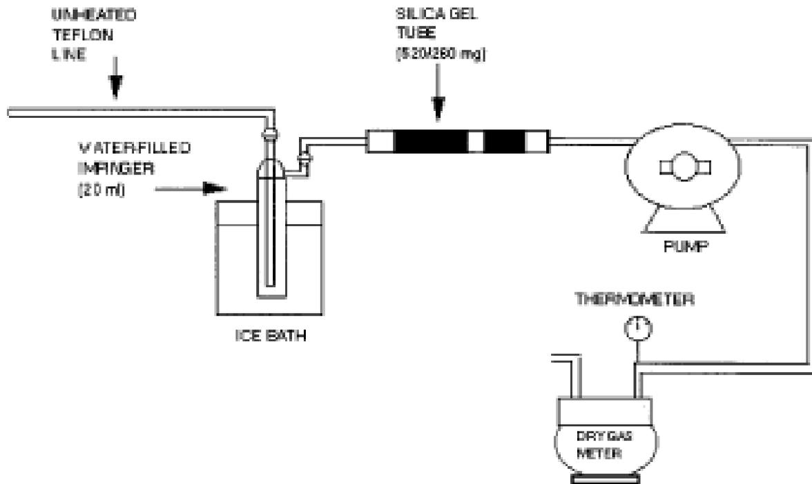
Figure 308.1. Sampling train schematic
