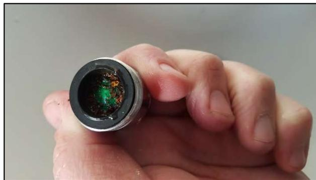
Picture of an aerator with particulate
