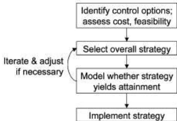
Fig. 3 Traditional framework for developing single-pollutant air quality attainment plans
