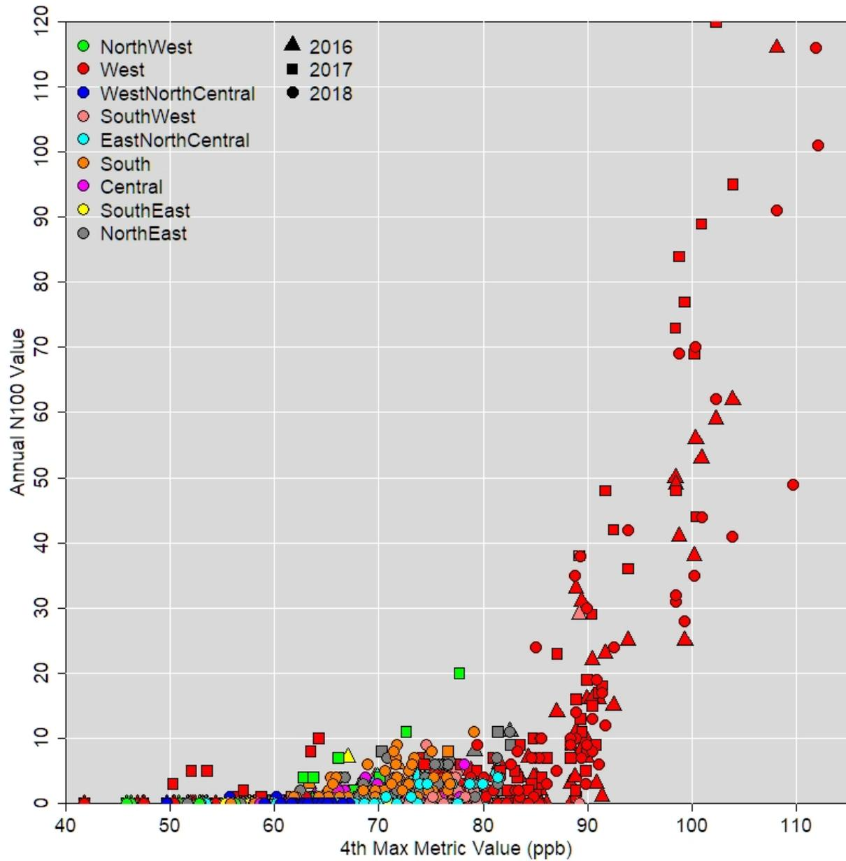
**Figure 4. Scatter plot of annual N100 values (y-axis) versus 4<sup>th</sup> max metric values (design values, x-axis) based on 2016-2018 monitoring data.**
