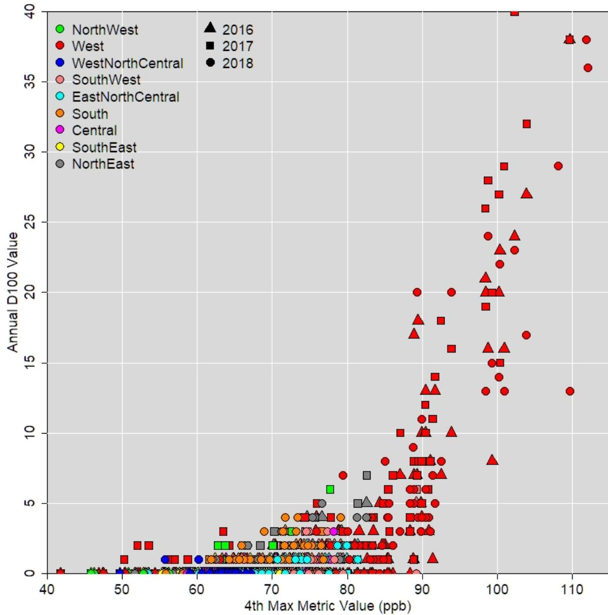
**Figure 5. Scatter plot of annual D100 values (y-axis) versus 4<sup>th</sup> max metric values (design values, x-axis) based on 2016-2018 monitoring data.**
