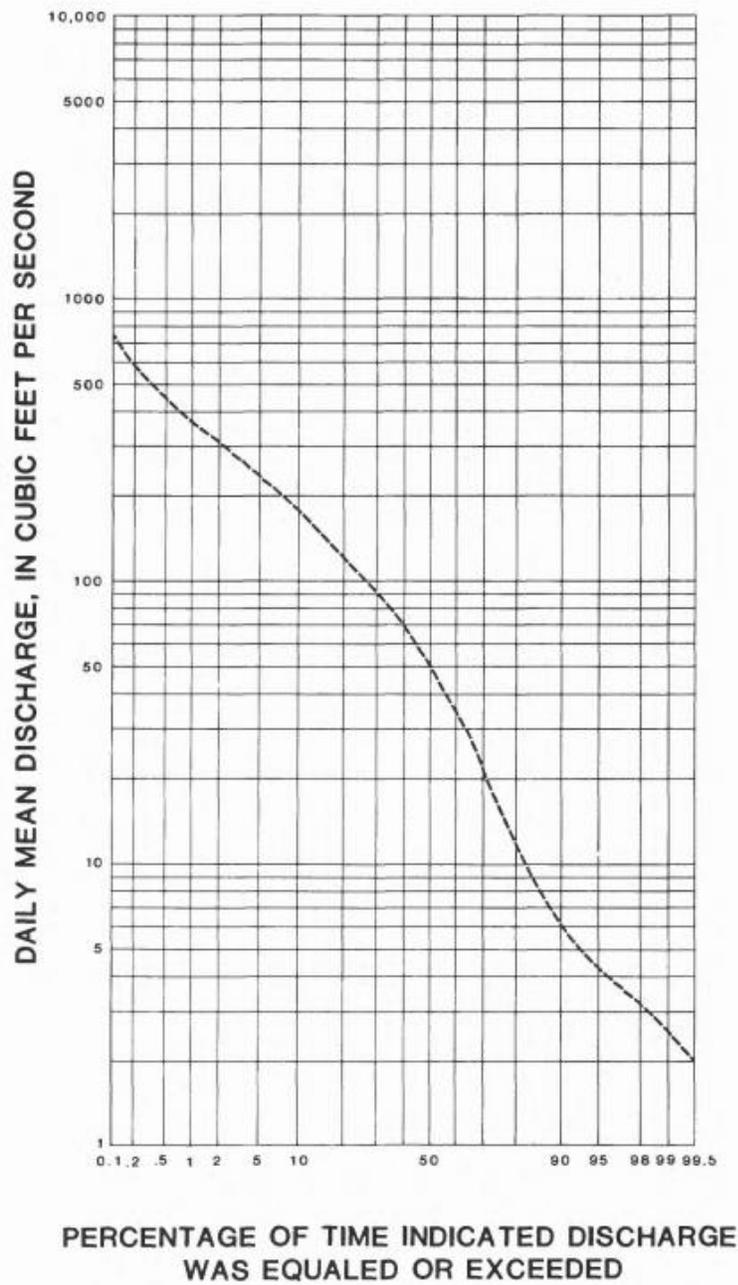
Figure 5.--Flow-duration curve for Wading River near Norton, Mass. (site 47), during 1955-81
