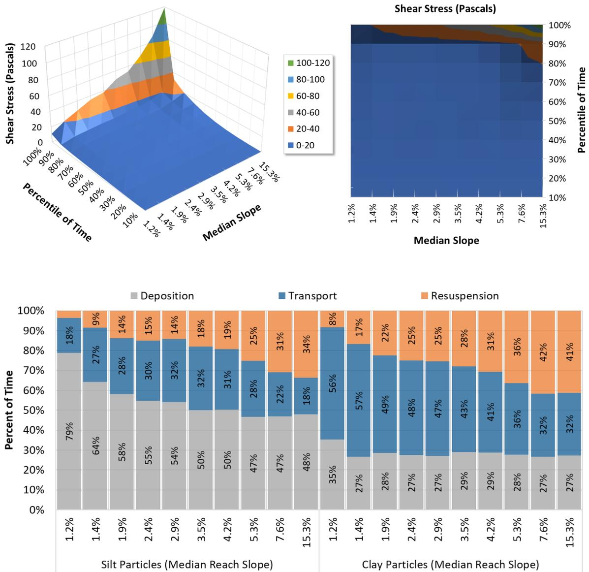
Figure 5. Post-processed shear stress output from LSPC. Top: Surface of stream bed boundary shear stress vs. slope and percent of the time (all modeled reaches). Bottom: Percent of time that silt and clay particles spend in the deposition, transport, and resuspension in model reach segments, as estimated from critical shear stress values.
