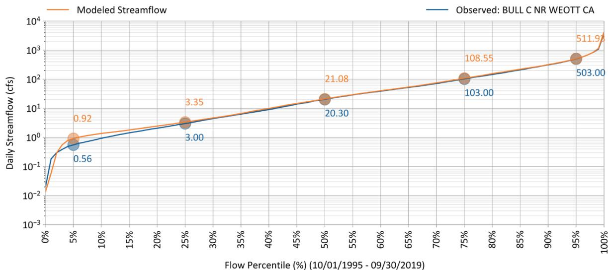
**Figure 6. Example calibration modeled vs. observed flow duration curve comparison.**
