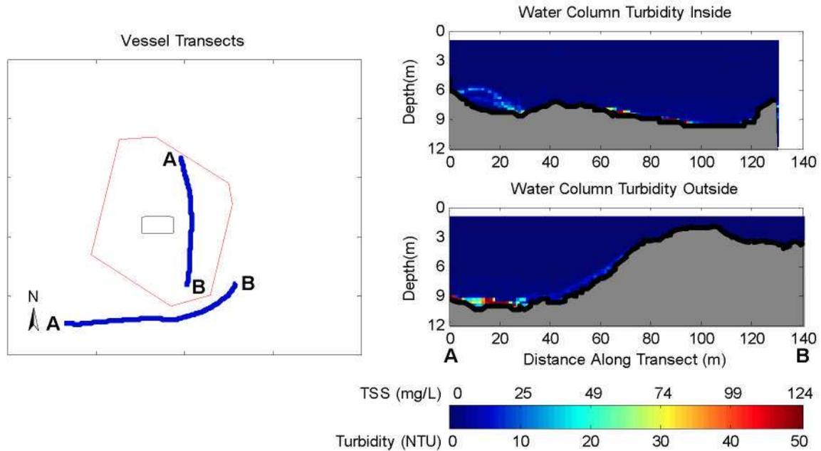
**Figure 5-1. Observations Before Release During July 8, 2009 Disposal into the New Bedford Harbor CAD Cell. The left panel shows concurrent inner and outer vessel transects. The right panel shows vertical slices of calibrated turbidity and TSS measured with ADCP along each vessel transect.**
