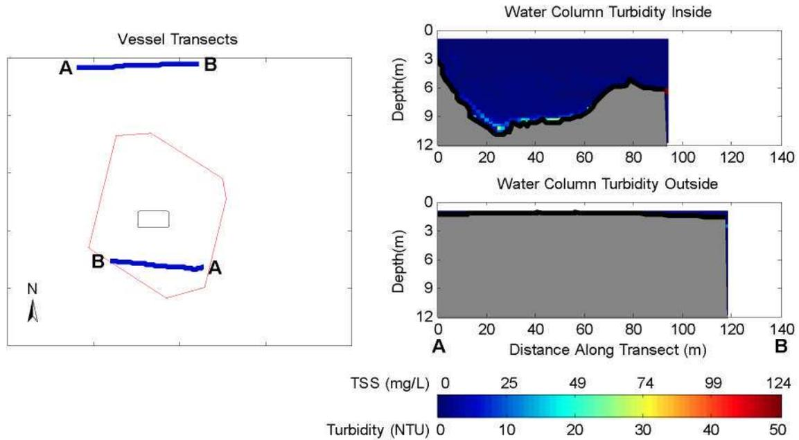
**Figure 1-5. Observations from 40 to 44 Minutes after Release During April 14, 2009 Disposal into the New Bedford Harbor CAD Cell. The left panel shows concurrent inner and outer vessel transects. The right panel shows vertical slices of calibrated turbidity and TSS measured with ADCP along each vessel transect.**
