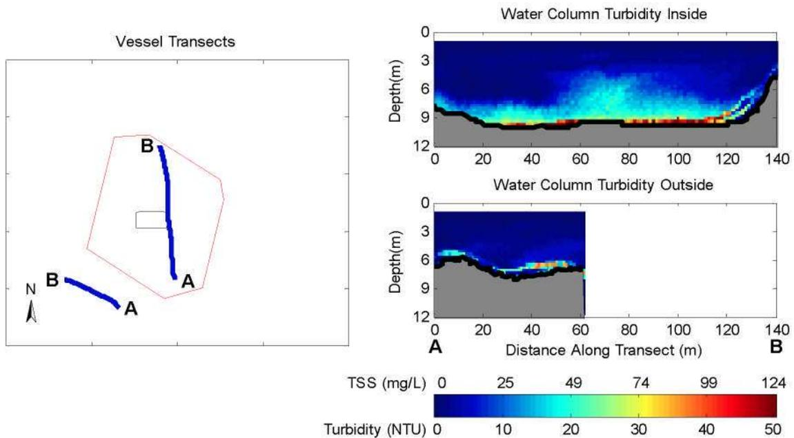
**Figure 3-4. Observations from 18 to 21 Minutes after Release During May 21, 2009 Disposal into the New Bedford Harbor CAD Cell. The left panel shows concurrent inner and outer vessel transects. The right panel shows vertical slices of calibrated turbidity and TSS measured with ADCP along each vessel transect.**
