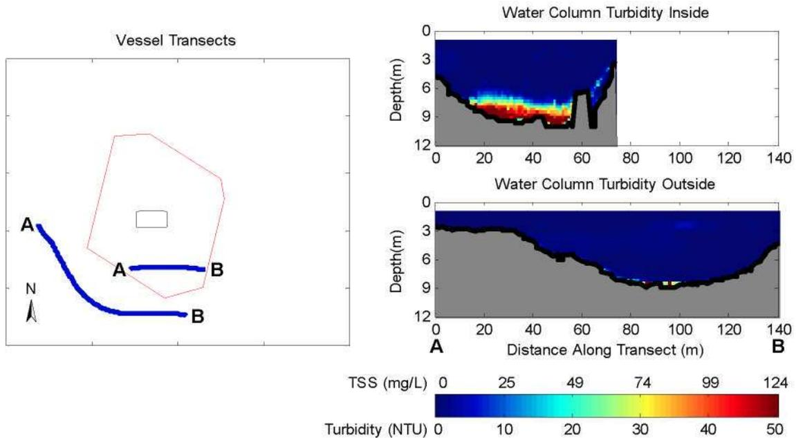
**Figure 3-2. Observations from 1 to 6 Minutes after Release During May 21, 2009 Disposal into the New Bedford Harbor CAD Cell. The left panel shows concurrent inner and outer vessel transects. The right panel shows vertical slices of calibrated turbidity and TSS measured with ADCP along each vessel transect.**
