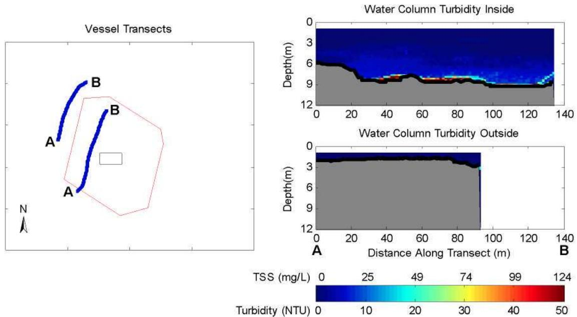
**Figure 5-7. Observations from 58 to 61 Minutes after Release During July 8, 2009 Disposal into the New Bedford Harbor CAD Cell. The left panel shows concurrent inner and outer vessel transects. The right panel shows vertical slices of calibrated turbidity and TSS measured with ADCP along each vessel transect.**
