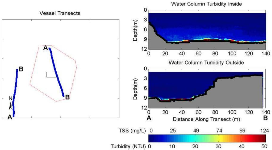
**Figure 3-7. Observations from 57 to 59 Minutes after Release During May 21, 2009 Disposal into the New Bedford Harbor CAD Cell. The left panel shows concurrent inner and outer vessel transects. The right panel shows vertical slices of calibrated turbidity and TSS measured with ADCP along each vessel transect.**
