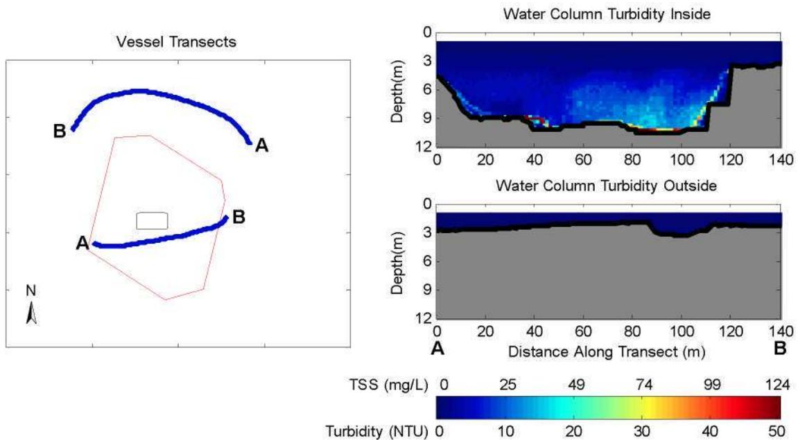
**Figure 4-6. Observations from 54 to 57 Minutes after Release During May 27, 2009 Disposal into the New Bedford Harbor CAD Cell. The left panel shows concurrent inner and outer vessel transects. The right panel shows vertical slices of calibrated turbidity and TSS measured with ADCP along each vessel transect.**
