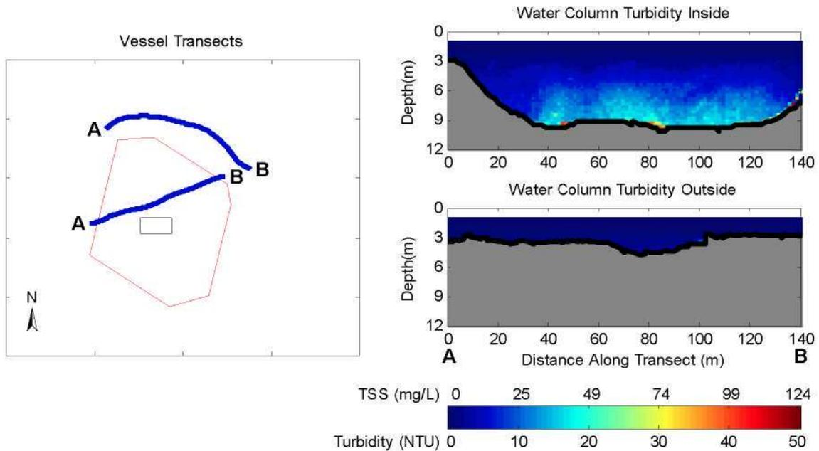
**Figure 4-5. Observations from 50 to 53 Minutes after Release During May 27, 2009 Disposal into the New Bedford Harbor CAD Cell. The left panel shows concurrent inner and outer vessel transects. The right panel shows vertical slices of calibrated turbidity and TSS measured with ADCP along each vessel transect.**
