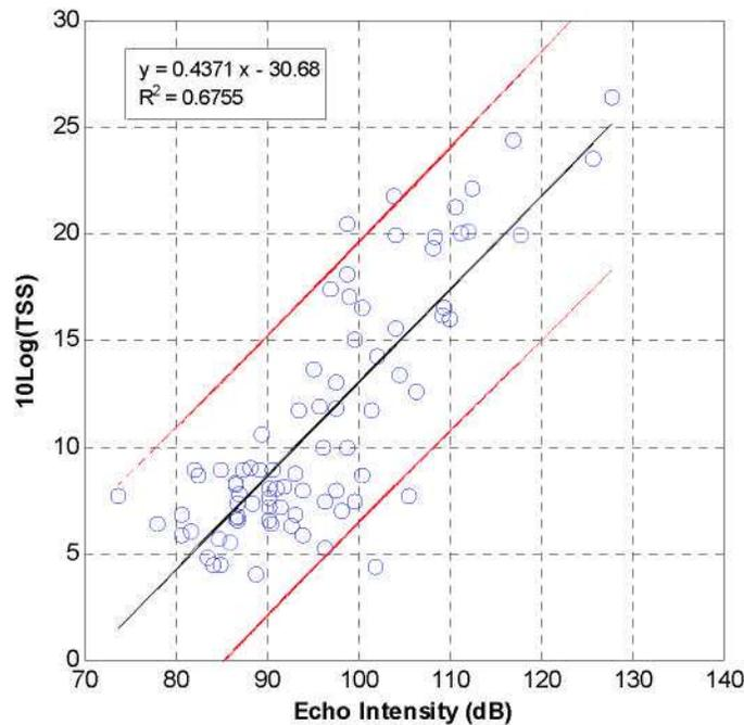
**Figure 5. Least Squares Regression Analysis of Total Suspended Solids (TSS) from Whole Water Samples Analyzed in the Laboratory versus ADCP Echo Intensity in Decibels (dB).**
