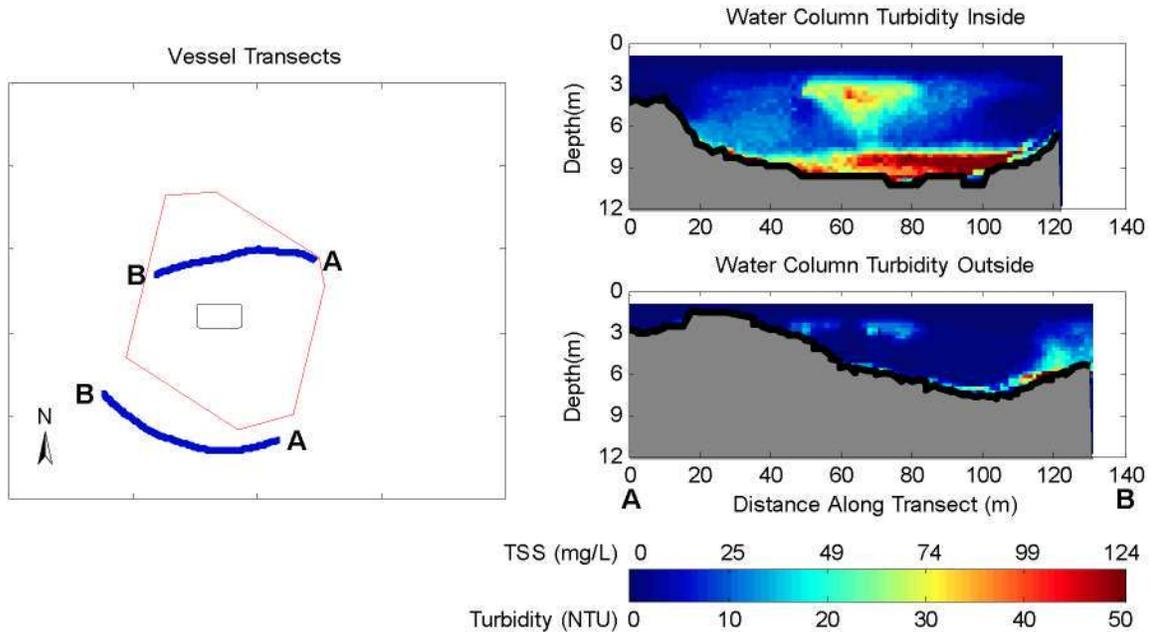
**Figure 3-3. Observations from 5 to 9 Minutes after Release During May 21, 2009 Disposal into the New Bedford Harbor CAD Cell. The left panel shows concurrent inner and outer vessel transects. The right panel shows vertical slices of calibrated turbidity and TSS measured with ADCP along each vessel transect.**
