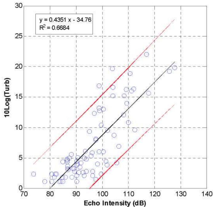
Figure 7. Least Squares Regression Analysis of Turbidity from Whole Water Samples Analyzed in the Laboratory versus ADCP Echo Intensity in Decibels (dB).
