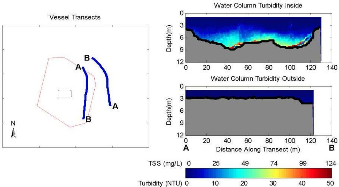
**Figure 4-4. Observations from 31 to 34 Minutes after Release During May 27, 2009 Disposal into the New Bedford Harbor CAD Cell. The left panel shows concurrent inner and outer vessel transects. The right panel shows vertical slices of calibrated turbidity and TSS measured with ADCP along each vessel transect.**
