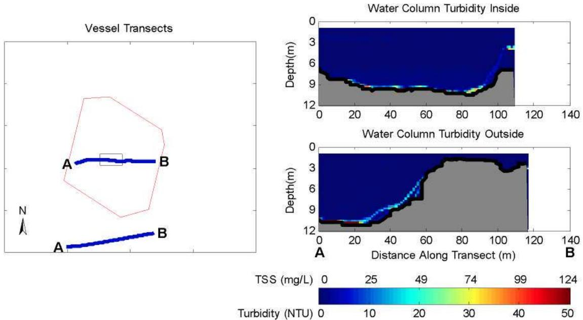
**Figure 3-1. Observations Before Release During May 21, 2009 Disposal into the New Bedford Harbor CAD Cell. The left panel shows concurrent inner and outer vessel transects. The right panel shows vertical slices of calibrated turbidity and TSS measured with ADCP along each vessel transect.**
