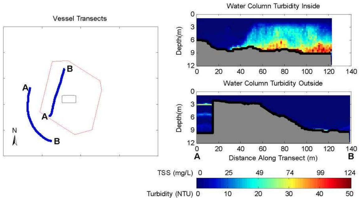
**Figure 5-2. Observations from 1 to 4 Minutes after Release During July 8, 2009 Disposal into the New Bedford Harbor CAD Cell. The left panel shows concurrent inner and outer vessel transects. The right panel shows vertical slices of calibrated turbidity and TSS measured with ADCP along each vessel transect.**
