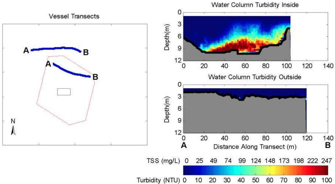
**Figure 4-3. Observations from 5 to 9 Minutes after Release During May 27, 2009 Disposal into the New Bedford Harbor CAD Cell. The left panel shows concurrent inner and outer vessel transects. The right panel shows vertical slices of calibrated turbidity and TSS measured with ADCP along each vessel transect. Note change in turbidity scale.**
