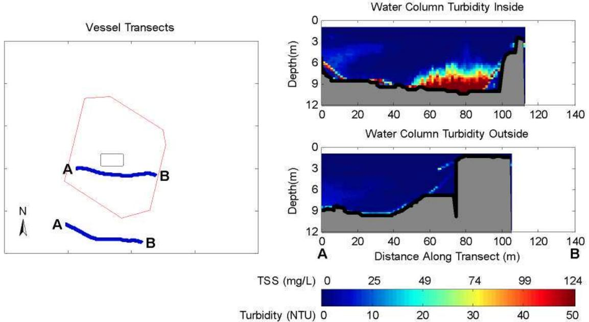
**Figure 2-2. Observations from 3 to 6 Minutes after Release During May 20, 2009 Disposal into the New Bedford Harbor CAD Cell. The left panel shows concurrent inner and outer vessel transects. The right panel shows vertical slices of calibrated turbidity and TSS measured with ADCP along each vessel transect.**
