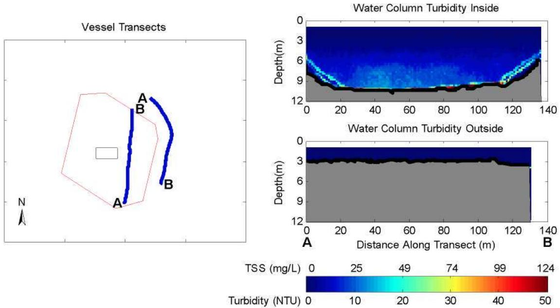
**Figure 4-7. Observations from 63 to 67 Minutes after Release During May 27, 2009 Disposal into the New Bedford Harbor CAD Cell. The left panel shows concurrent inner and outer vessel transects. The right panel shows vertical slices of calibrated turbidity and TSS measured with ADCP along each vessel transect.**
