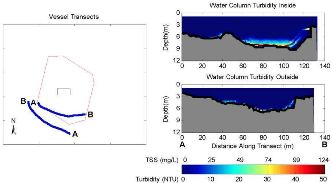
**Figure 5-3. Observations from 9 to 16 Minutes after Release During July 8, 2009 Disposal into the New Bedford Harbor CAD Cell. The left panel shows concurrent inner and outer vessel transects. The right panel shows vertical slices of calibrated turbidity and TSS measured with ADCP along each vessel transect.**
