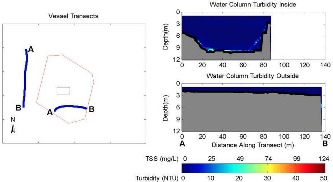
**Figure 2-1. Observations Before Release During May 20, 2009 Disposal into the New Bedford Harbor CAD Cell. The left panel shows concurrent inner and outer vessel transects. The right panel shows vertical slices of calibrated turbidity and TSS measured with ADCP along each vessel transect.**
