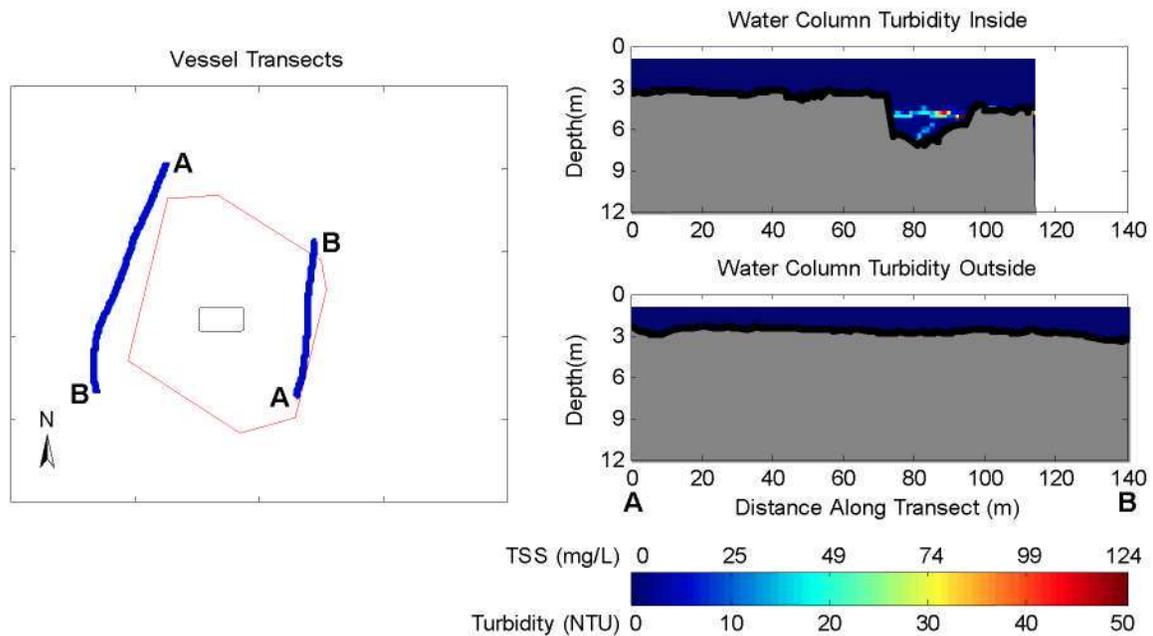
**Figure 5-4. Observations from 15 to 18 Minutes after Release During July 8, 2009 Disposal into the New Bedford Harbor CAD Cell. The left panel shows concurrent inner and outer vessel transects. The right panel shows vertical slices of calibrated turbidity and TSS measured with ADCP along each vessel transect.**
