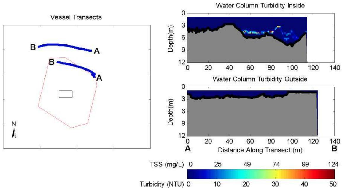
**Figure 1-1. Observations Before Release During April 14, 2009 Disposal into the New Bedford Harbor CAD Cell. The left panel shows concurrent inner and outer vessel transects. The right panel shows vertical slices of calibrated turbidity and TSS measured with ADCP along each vessel transect.**
