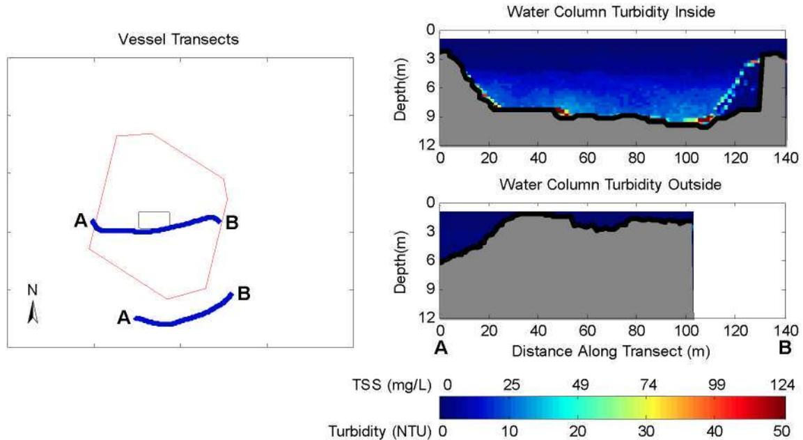
**Figure 2-7. Observations from 84 to 87 Minutes after Release During May 20, 2009 Disposal into the New Bedford Harbor CAD Cell. The left panel shows concurrent inner and outer vessel transects. The right panel shows vertical slices of calibrated turbidity and TSS measured with ADCP along each vessel transect.**
