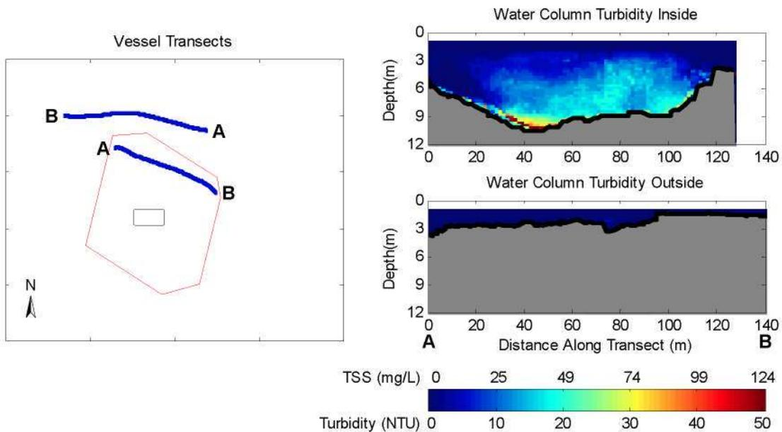
**Figure 1-2. Observations from 8 to 11 Minutes after Release During April 14, 2009 Disposal into the New Bedford Harbor CAD Cell. The left panel shows concurrent inner and outer vessel transects. The right panel shows vertical slices of calibrated turbidity and TSS measured with ADCP along each vessel transect.**
