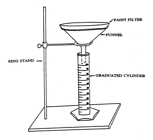
Figure 1. Paint filter test apparatus.
