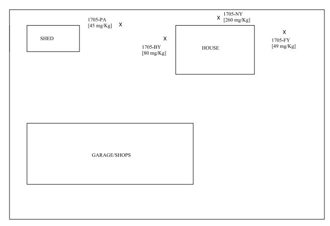
X: Sample Location, Approximate [- mg/Kg]: ICP Lead in Soils Analytical Result
