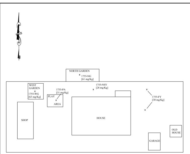
X: Sample Location, Approximate [- mg/Kg]: ICP Lead in Soils Analytical Result
