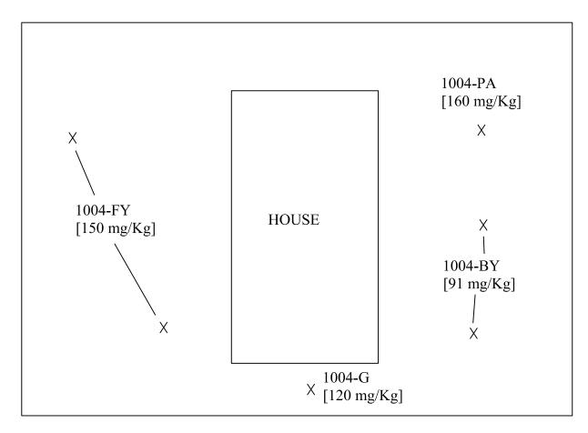
X: Sample Location, Approximate [- mg/Kg]: ICP Lead in Soils Analytical Result
