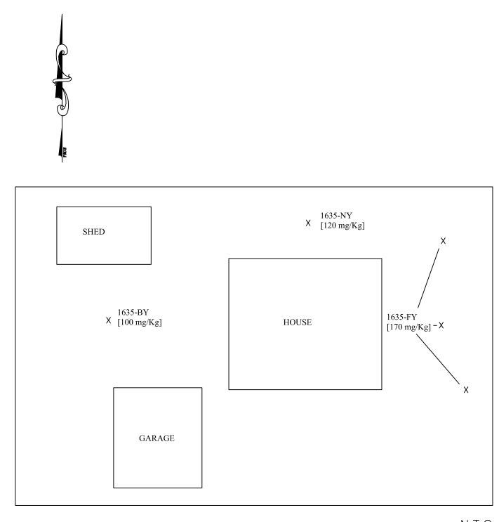
X: Sample Location, Approximate [- mg/Kg]: ICP Lead in Soils Analytical Result
