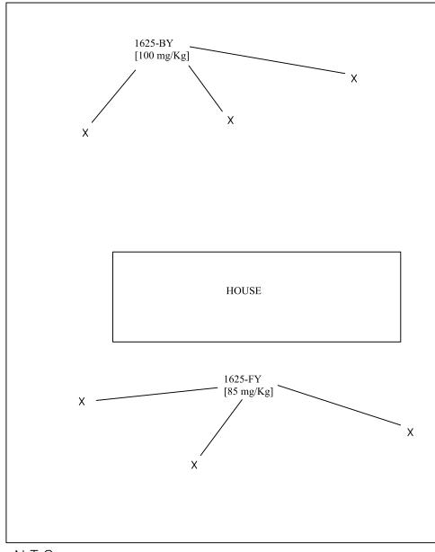
X: Sample Location, Approximate [- mg/Kg]: ICP Lead in Soils Analytical Result
