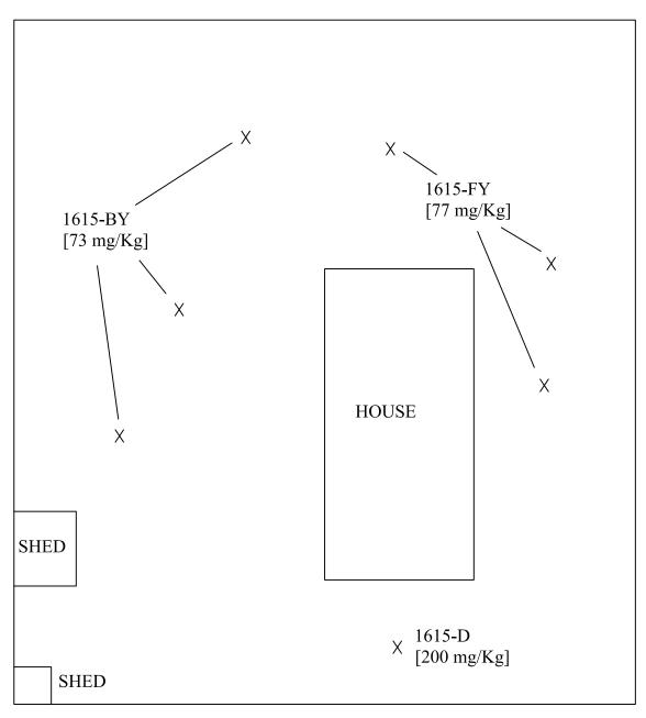
X: Sample Location, Approximate [- mg/Kg]: ICP Lead in Soils Analytical Result
