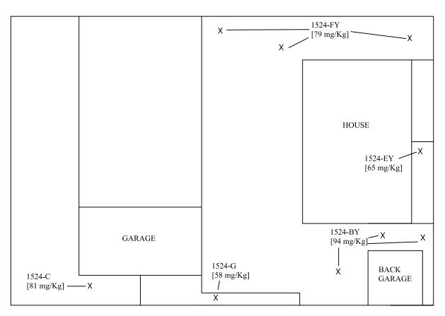
X: Sample Location, Approximate [- mg/Kg]: ICP Lead in Soils Analytical Result
