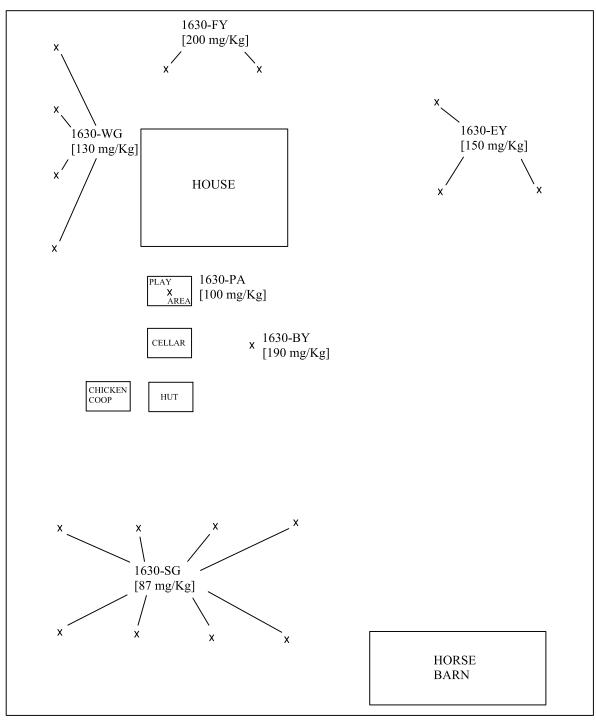
X: Sample Location, Approximate [- mg/Kg]: ICP Lead in Soils Analytical Result
