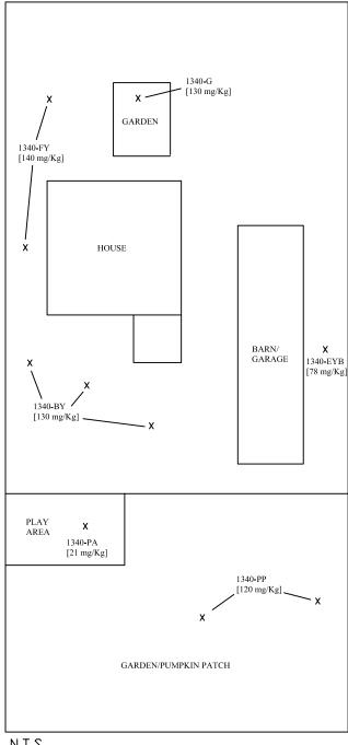
X: Sample Location, Approximate [- mg/Kg]: ICP Lead in Soils Analytical Result
