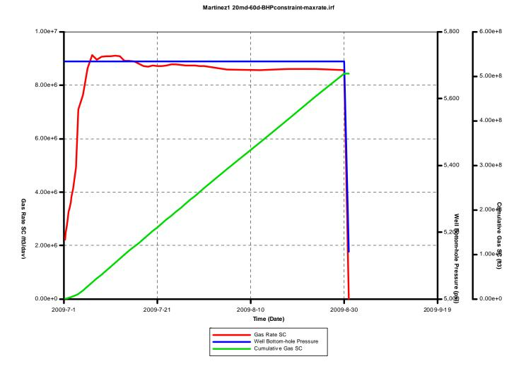
Figure N-4 Base Case Injection Profile into the 20 mD Sand
