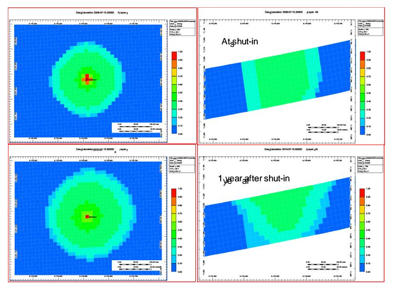
Figure N-9 CO<sub>2</sub> Plume Maps in the 20md-6,000ton Case
