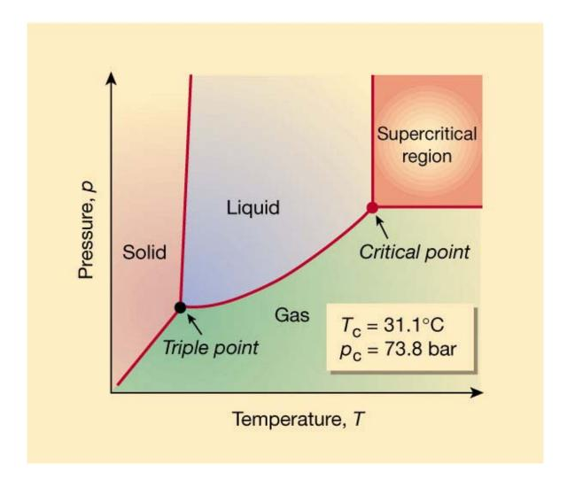
Figure P-1 Carbon Dioxide Phase Diagram
