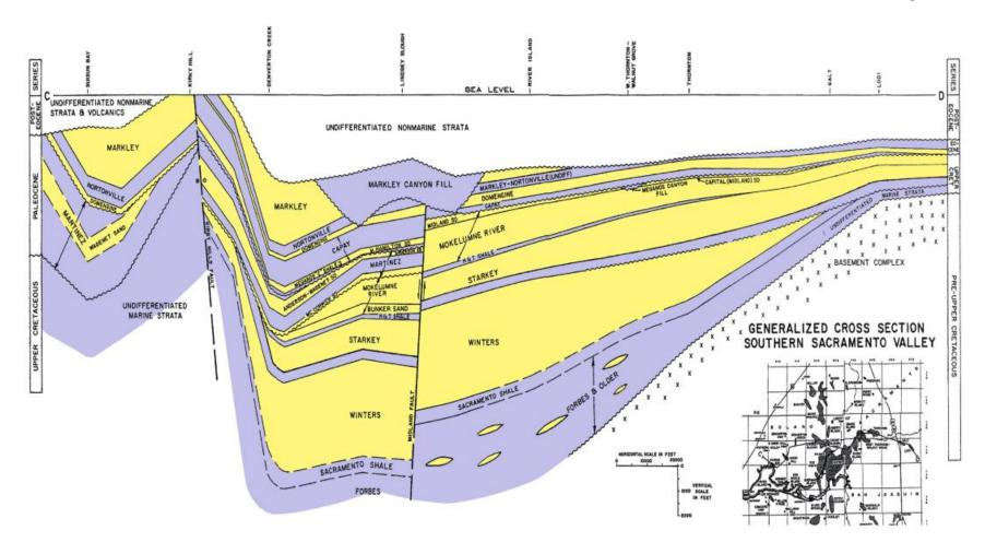
Figure F-3 Generalized Cross Section Through the Southern Sacramento Valley (modified from DOGGR, 1983)
