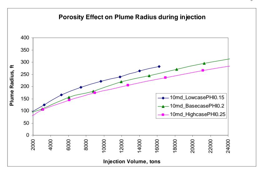
Figure N-12 Porosity Effect on CO<sub>2</sub> Plume Size during Injection
