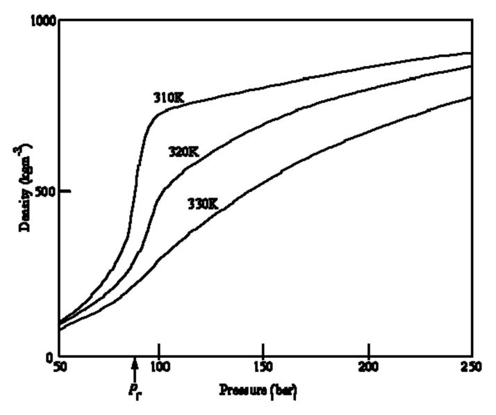
Figure P-2 Variation of Carbon Dioxide Density with Pressure and Temperature (<a href="www.chem.leeds.ac.uk/People/CMR/props.html">www.chem.leeds.ac.uk/People/CMR/props.html</a>).
