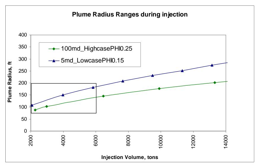
Figure N-13 CO<sub>2</sub> Plume Radius Ranges during Injection
