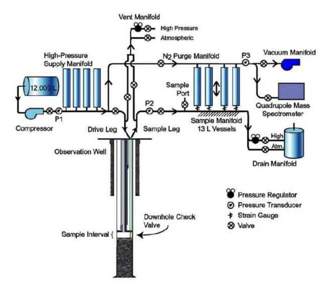
Figure P-3 U-tube Sampler Configuration Used to Collect Fluid Samples.
