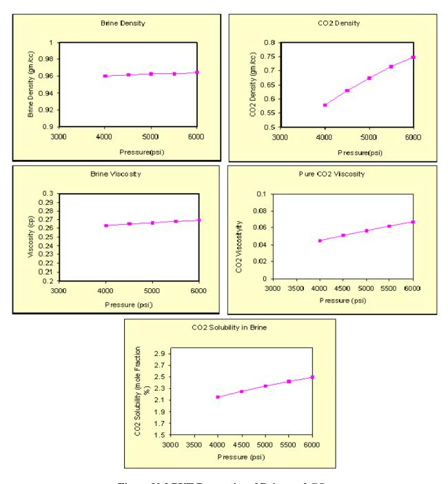
Figure N-3 PVT Properties of Brine and CO<sub>2</sub>
