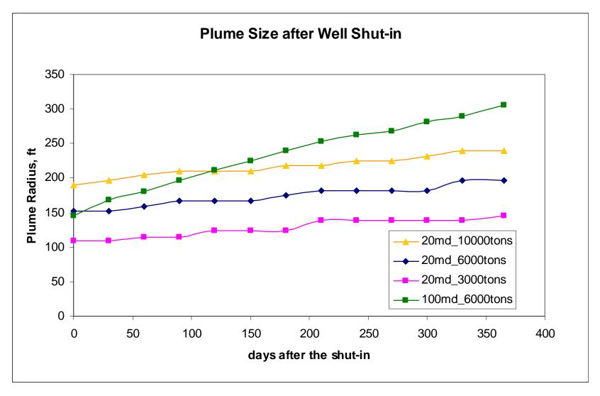
Figure N-7 CO<sub>2</sub> Plume Size Following Cessation of Injection
