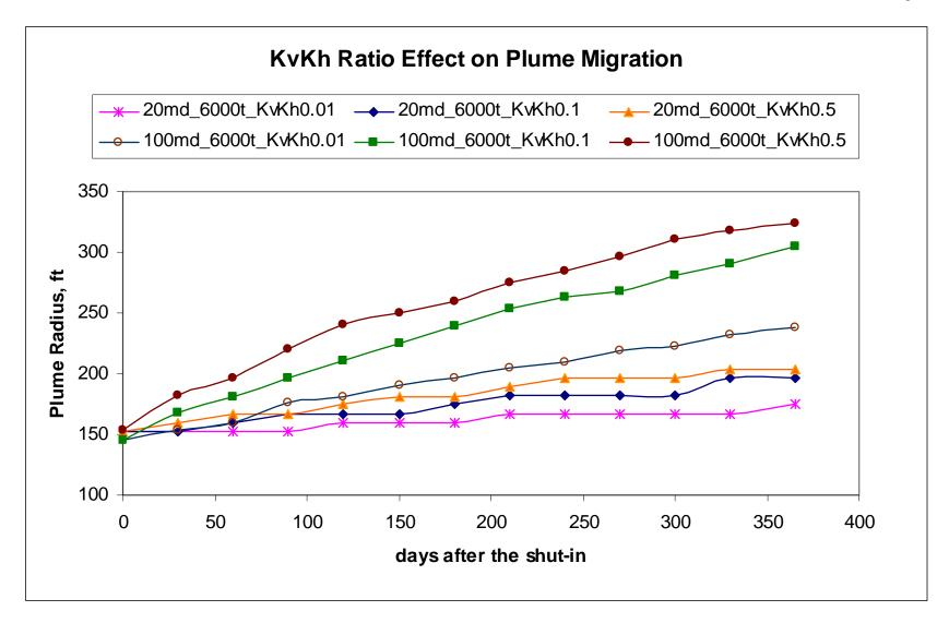
Figure N-11 Vertical Permeability Effect on CO<sub>2</sub> Plume Size
