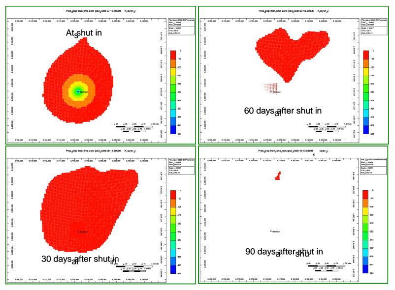
Figure N-14 Pressure Maps in the 20md-6,000ton Case
