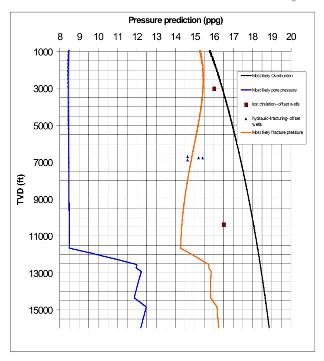
**Figure G-2 Pore and Fracture Pressure Predictions**
