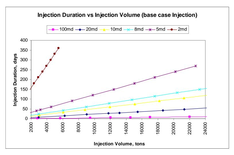
Figure N-5 Predicted Pilot Injection Duration (Base Case Injectivity)
