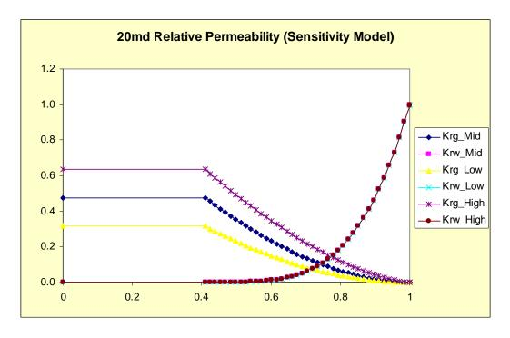
Figure N-1b Relative Permeability Sensitivity Model (20 mD rock)
