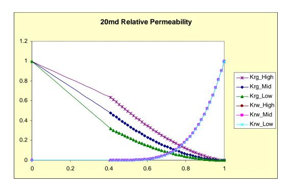
Figure N-1a CO<sub>2</sub>-Water Relative Permeability Model (20 mD rock)
