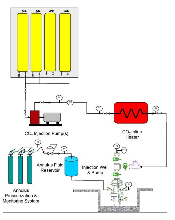
Figure K-1 Proposed Temporary CO<sub>2</sub> Surface Facilities.
