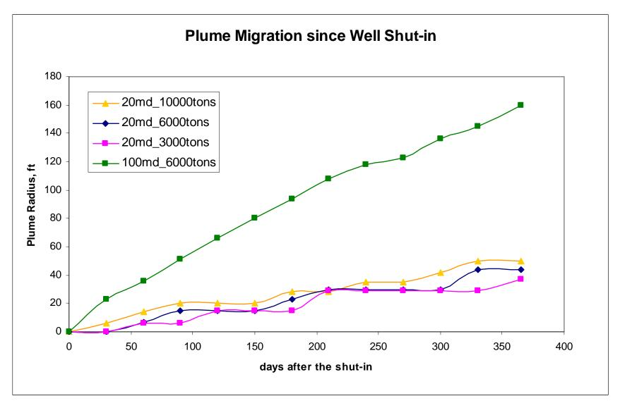
Figure N-8 CO<sub>2</sub> Plume Incremental Movement Following Cessation of Injection
