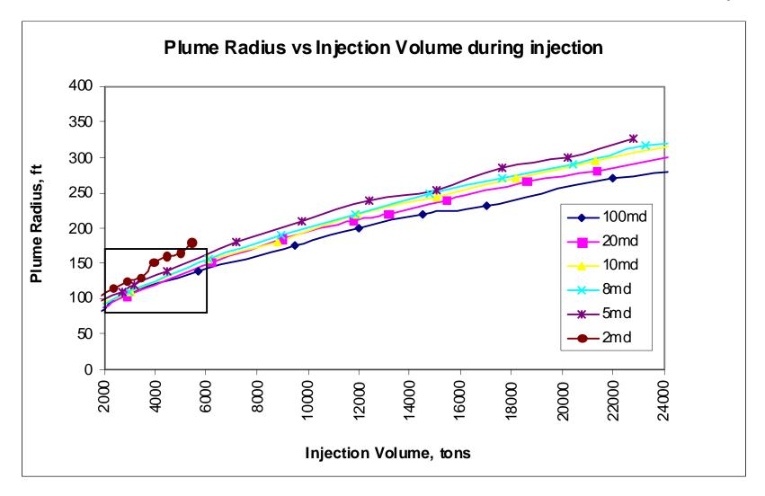
Figure N-6 CO<sub>2</sub> Plume Size during Injection
